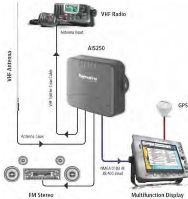
Fig. 2. AIS configuration [2]
