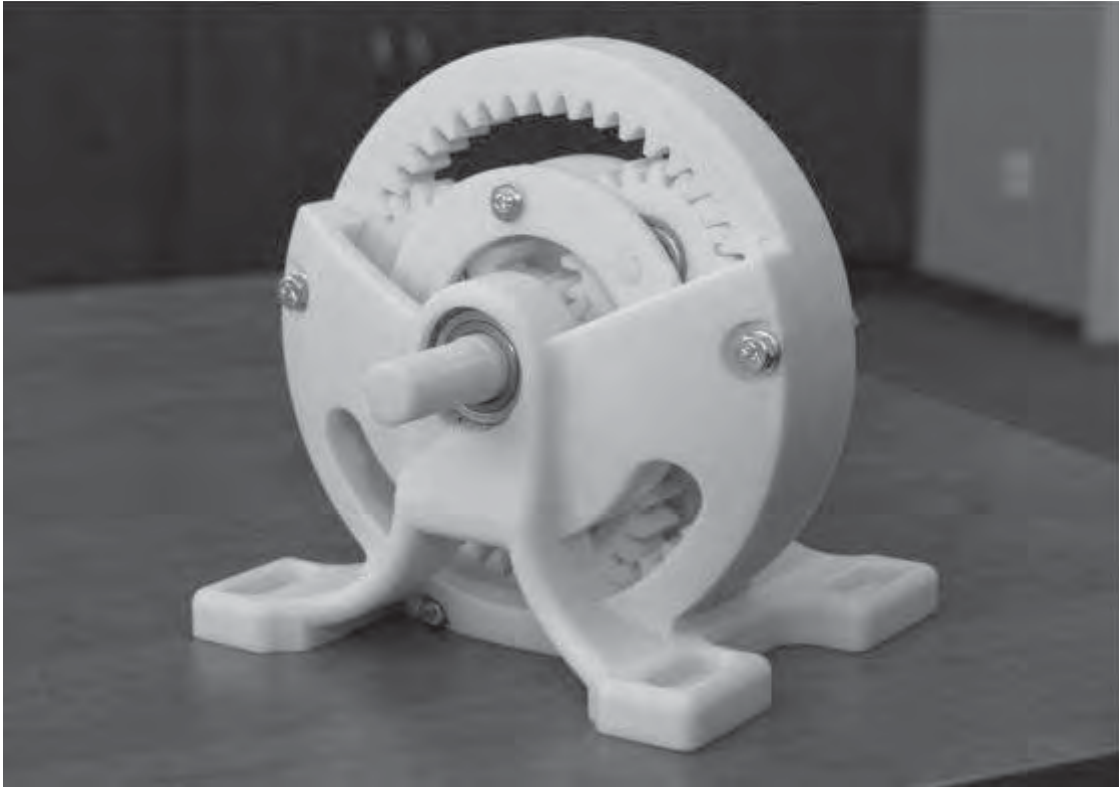
Fig. 6. A model of the research gear made by means of FDM
