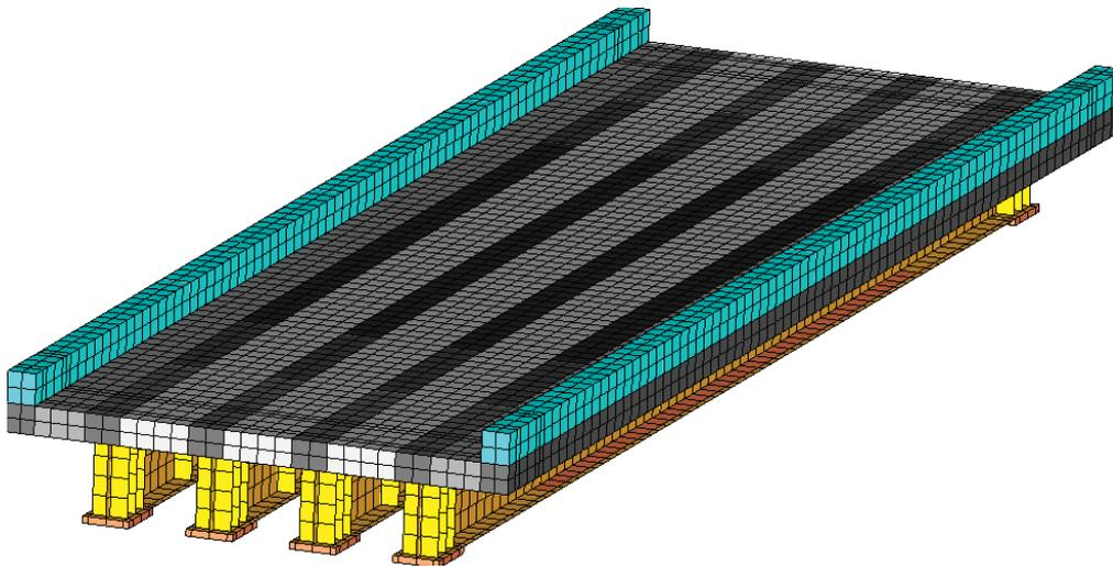
Fig. 6. The FE model of the KNI 140070 viaduct superstructure
