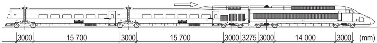
Fig. 1. A schematic diagram of the KTX train [16]
