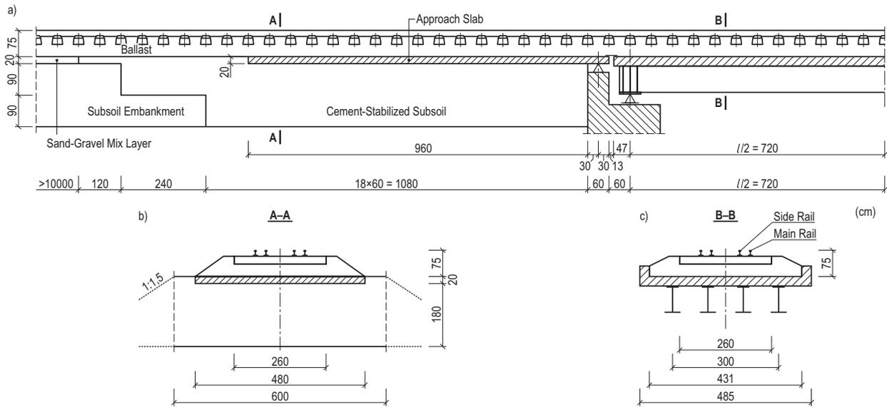
Fig. 3. The modernized ballasted track in the KNI 140070 bridge area: a) a longitudinal section; b) a cross-section in the approach zone; c) a cross-section over the bridge span
