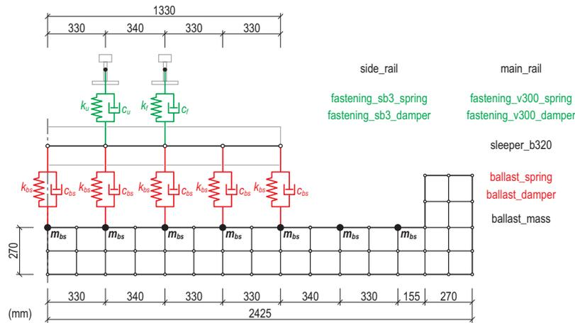
Fig. 7. The KNI 140070 viaduct's platform cross-section. The FE model of the track over the bridge platform (the components marked with different colours)
