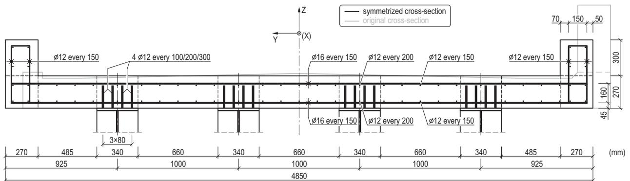
Fig. 4. The original and symmetrised cross-sections of the KNI 140070 viaduct and the symmetrised reinforcement
