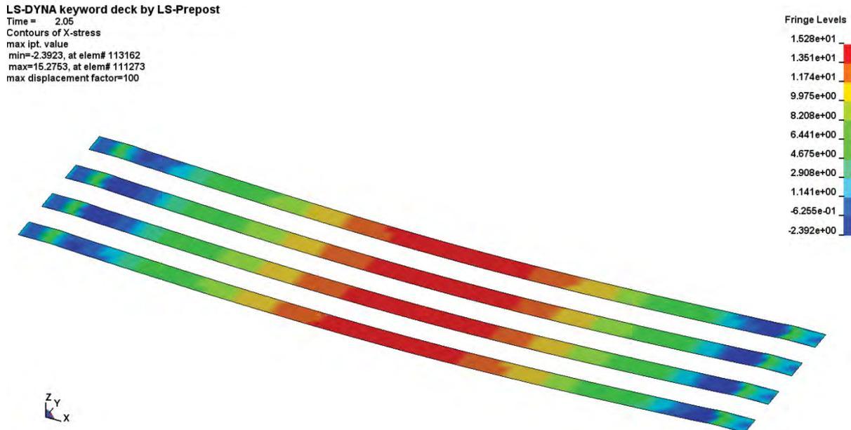
Fig. 10. Contours of the longitudinal normal stresses  $\sigma_x$  [MPa] in the bottom flanges of the main beams at  $t = 2.05$  sec (the scale coefficient 100x for displacements)
