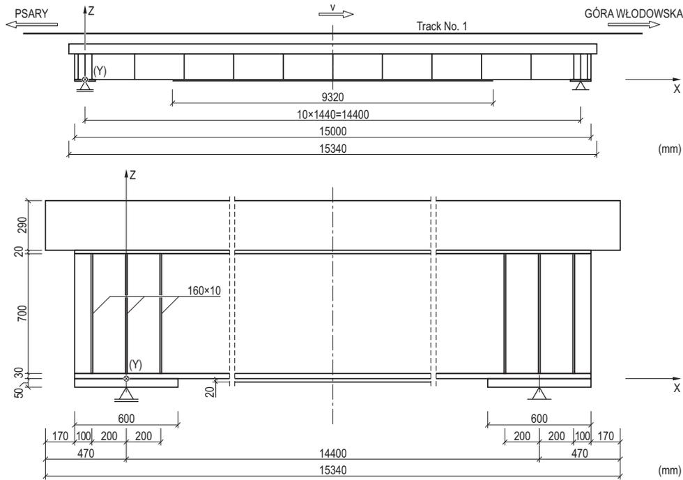
Fig. 2. The longitudinal sections of the KNI 140070 viaduct in the XZ plane
