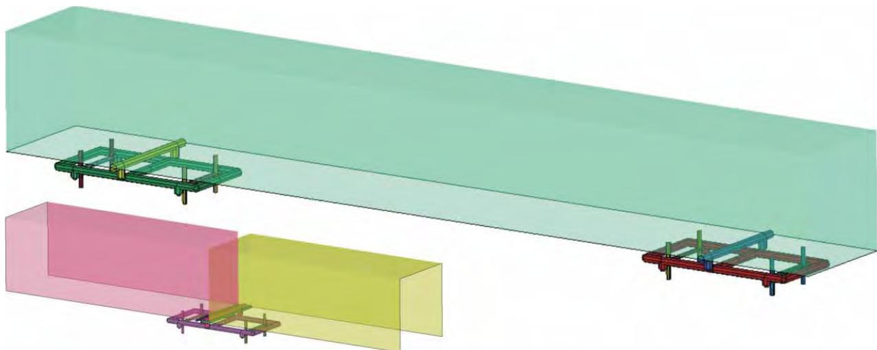
Fig. 8. A numerical model of the KTX units with classic and Jacob's bogies
