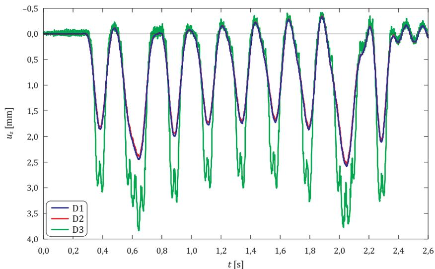
Fig. 9. Time-histories of selected vertical displacements at the midspan: D1 – the central point of the bottom flange of the internal main beam; D2 – the central point of the bottom flange of the external main beam; D3 – the main rail
