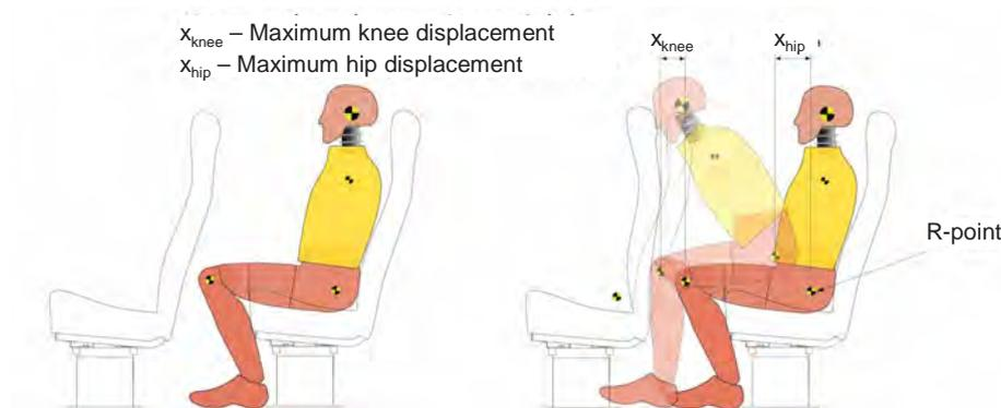
Fig. 5. Dummies ready for the test and knee and hip displacement measures
