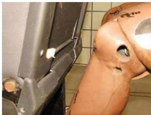
Fig. 15. Visible damage to the backrest caused by the Hybrid dummy's knees impact
