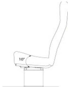
Fig. 7. Seat inclination angle
