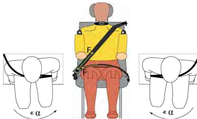
Fig. 12. Lower torso (hips) rotation depending on belt orientation and seat position
