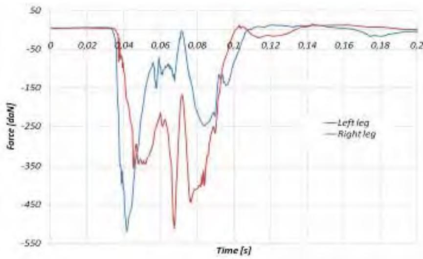
Fig. 14. Force acting on the thighs of an unsecured dummy, seat angle 10°
