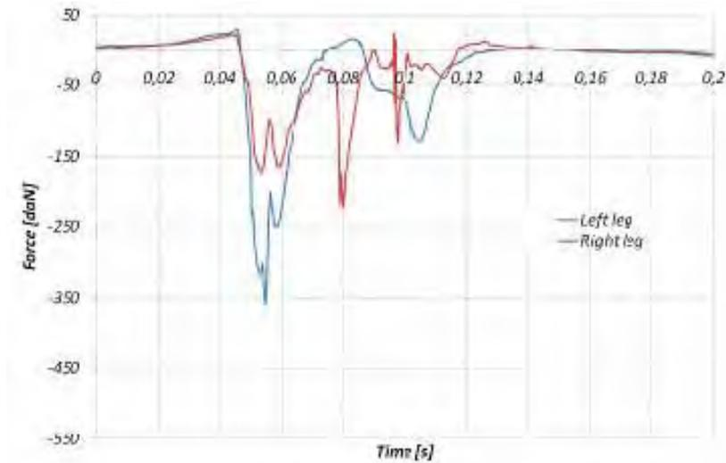
Fig. 11. Force exerted on thighs of the dummy secured with a 3-point belt, seat angle  $10^\circ$
