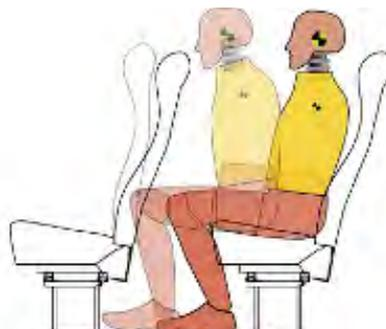
Fig. 9. Dummy secured with a 2-point belt, seat angle 10°
