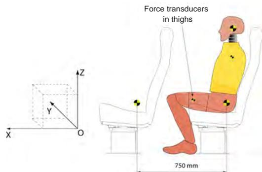
Fig. 2. Sensor positions in the Hybrid dummy and the frame of reference for the transducer axes in the initial (static) state
