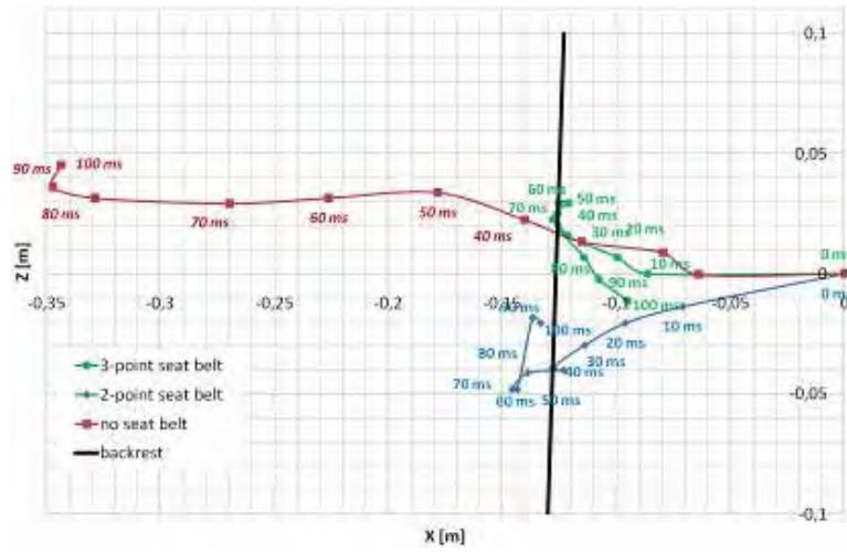
Fig. 6. Knee movement (displacement) trajectories during an impact at 30 km/h; seat angle 10°
