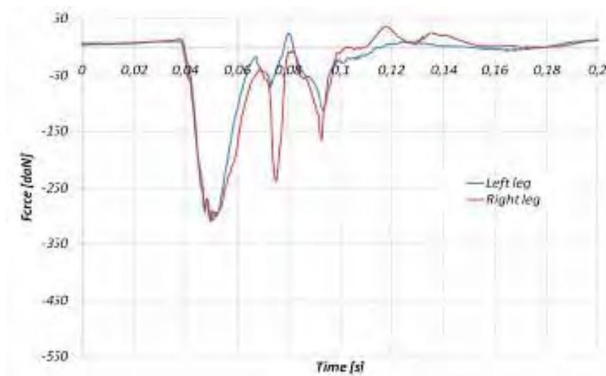
Fig. 13. Force acting on the thighs of a dummy secured with a 2-point belt, seat angle  $10^\circ$
