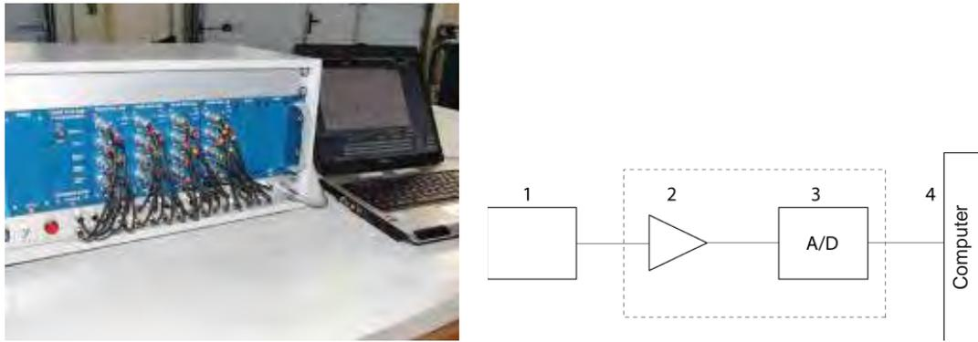
Fig. 4. TDAS DTS ProLab digital recorder and measuring system diagram: 1 – Force and acceleration transducers, 2 – power supply, measuring amplifier, 3 – Analog/digital converter, 4 – PC with TDAS Control registration software
