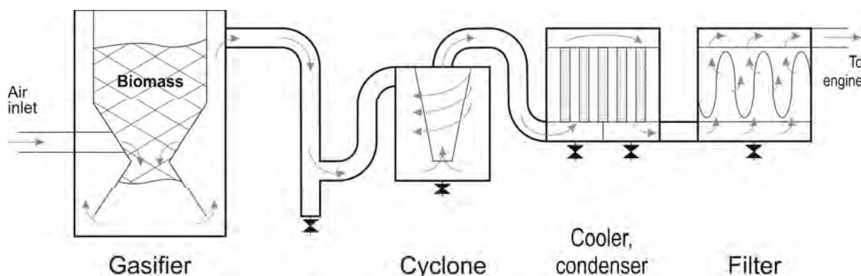
Fig. 4. Typical gas conditioning setup
