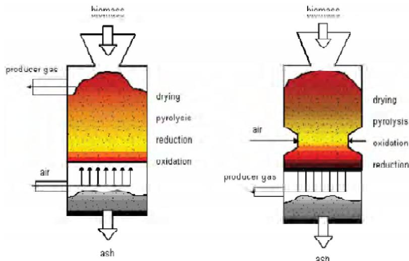
Fig. 3. Scheme of updraft and down draft gasifier with enhanced reaction zones
