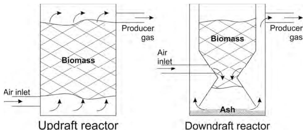
Fig.2. Scheme of updraft and down draft gasifier
