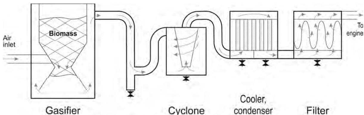
Fig. 4. Typical gas conditioning setup
