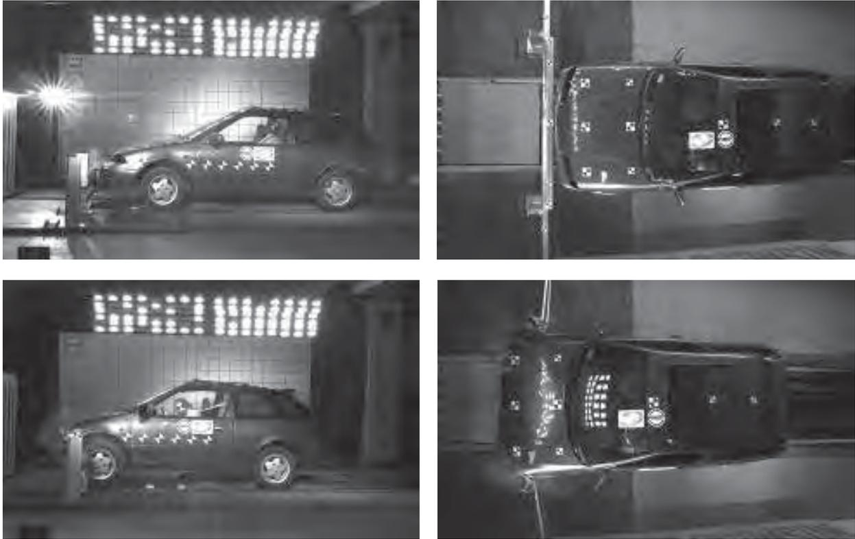
Fig. 4. The crash test course registered with the use of two synchronized cameras designed for fast shooting
