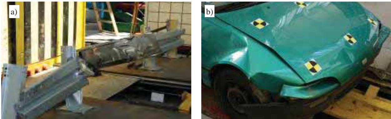
Fig. 5. Deformation of the tested protective road barrier type 1A (a) and Suzuki Swift car's deformation (b)
