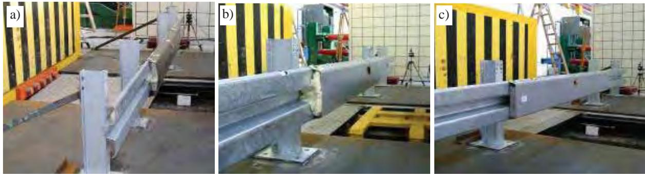
Fig. 3. Road barrier with a panel type 1A (a), 1B (b), 1BL (c)
