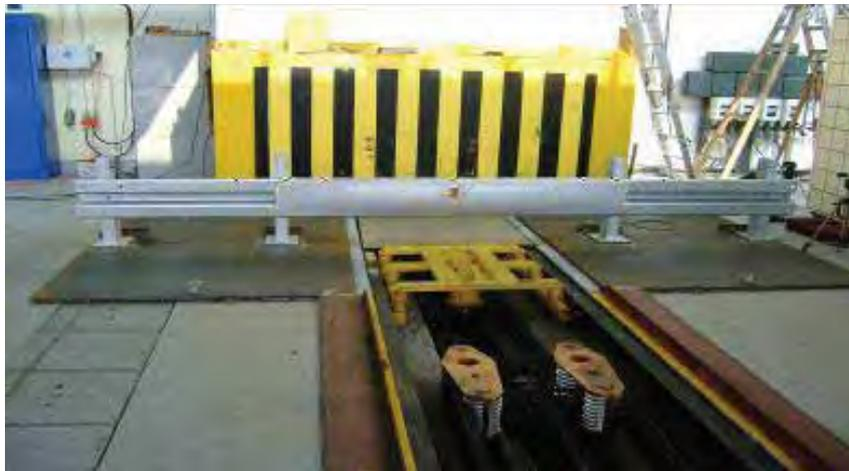
*Fig. 1. Stand for vehicle crash tests with a modified road barrier in PIMOT's Vehicle Safety Laboratory*
