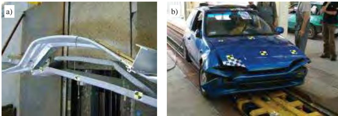
Fig. 11. Deformation of the tested protective road barrier type 1AL (a) and Suzuki Swift car's deformation (b)
