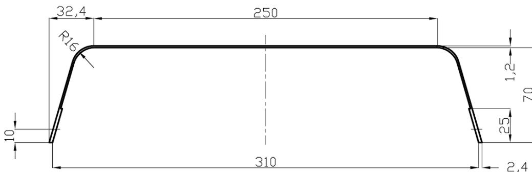
*Fig. 2. The scheme of a protective panel with the casing of trapezoid form with the height of 70 mm*
