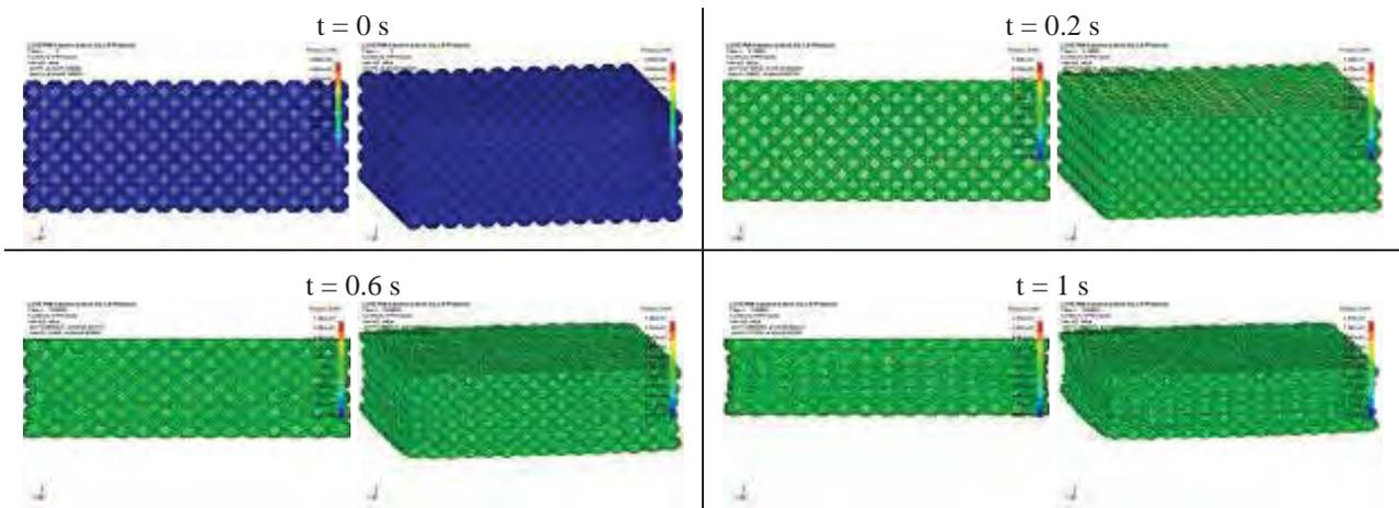
Fig. 4. Pressure distribution for compression test of aluminium foam microstructure FE model
