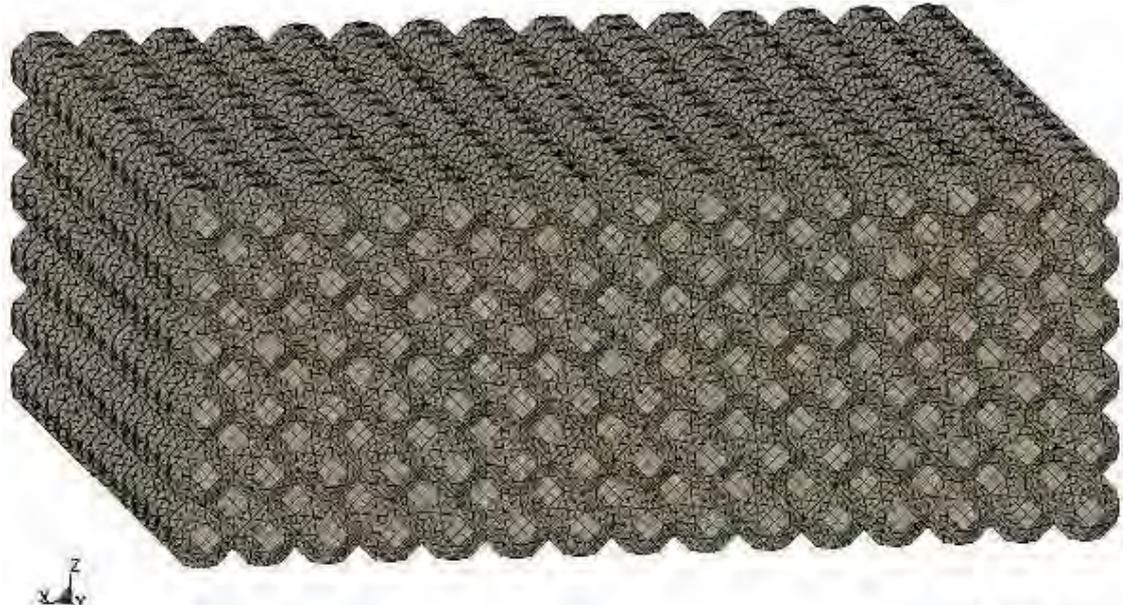
Fig. 1. Numerical model of closed-cell aluminium foam microstructure
