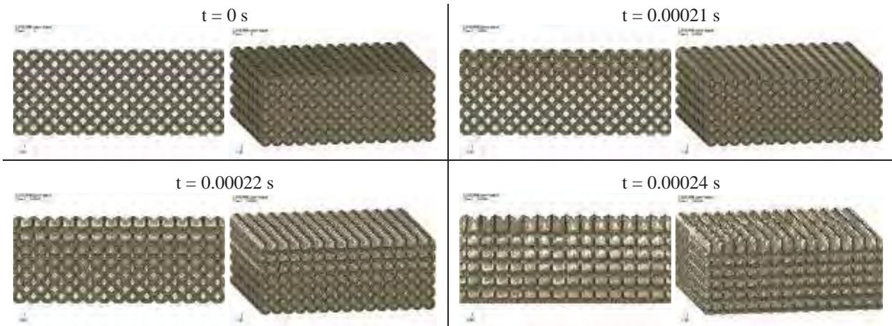
Fig. 7. Deformations for blast loading of aluminium foam microstructure FE model
