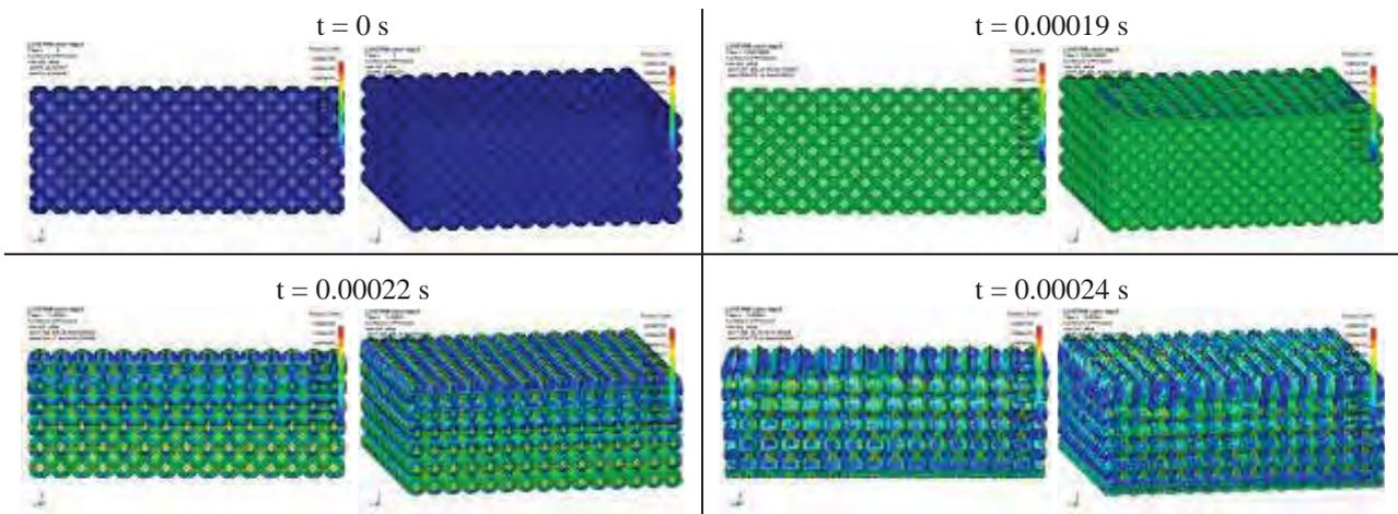
Fig. 8. Pressure distribution for blast loading of aluminium foam microstructure FE model
