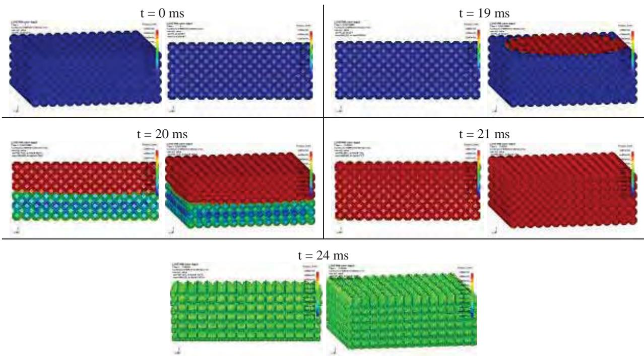
Fig. 8. Effective stress distribution for blast loading of aluminium foam microstructure FE model
