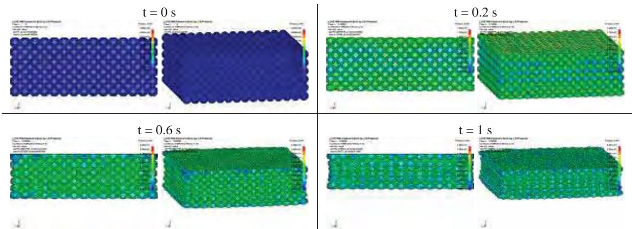
Fig. 5. Effective stress distribution for compression test of aluminium foam microstructure FE model
