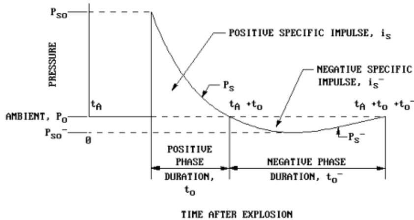
Fig. 6. Pressure-time evolution during blast load
