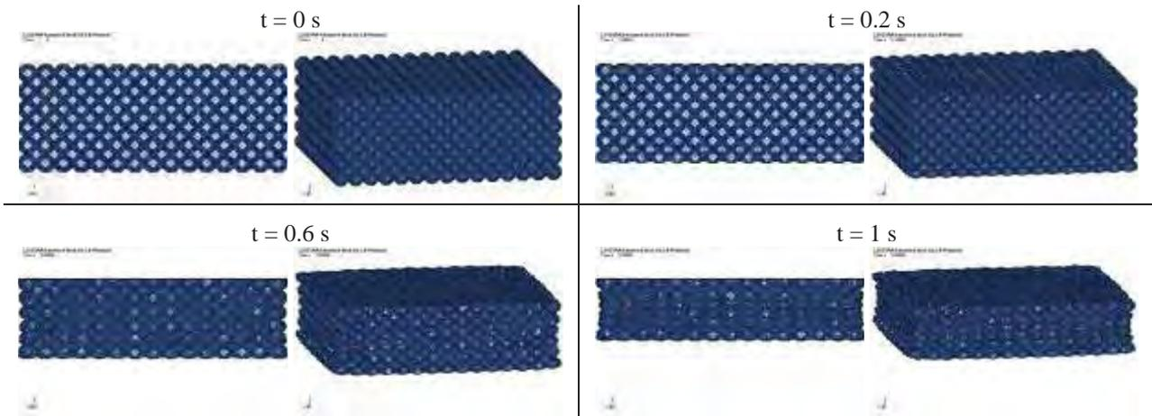
Fig. 3. Deformations for compression test of aluminium foam microstructure FE model
