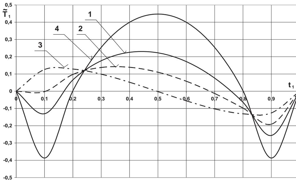
Fig. 5. Change the dimensionless friction forces  $\tilde{T}_1$  in the time  $t_1$  by velocity perturbations: 1)  $V_{10}=0.05$ ,  $V_{1h}=0$ , 2)  $V_{10}=0.05$ ,  $V_{1h}=0.025$ , 3)  $V_{10}=0.05$ ,  $V_{1h}=0.05$ , 4)  $V_{10}=0.05$ ,  $V_{1h}=-0.05$
