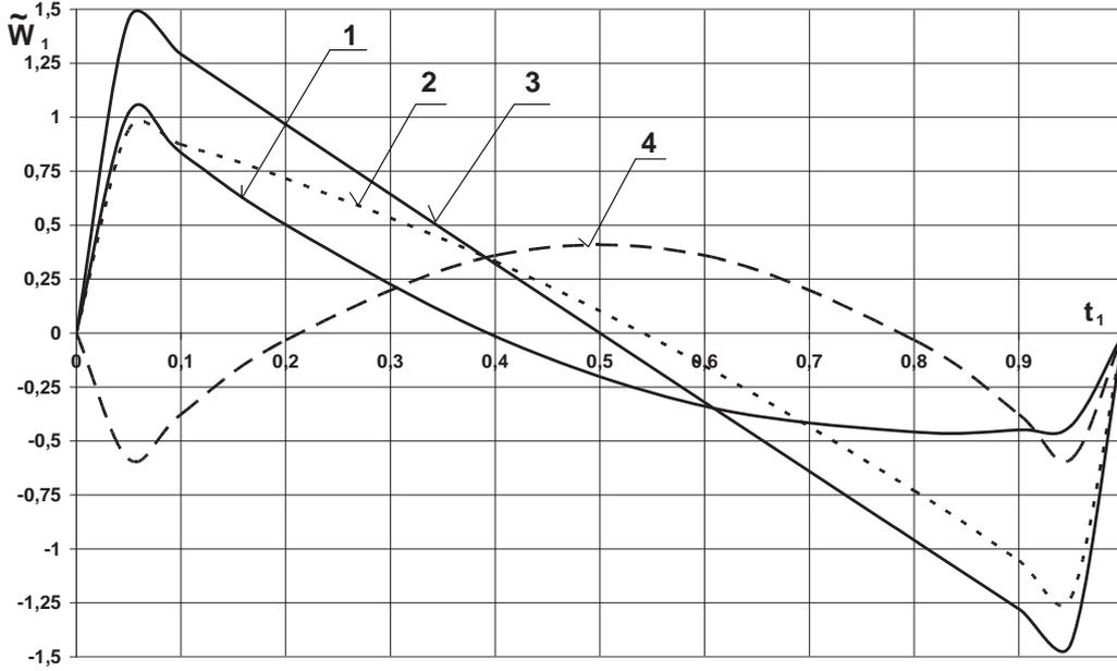
Fig. 3. Change the dimensionless capacity forces  $\tilde{W}_1$  in the time  $t_1$  by velocity perturbations: 1)  $V_{10}=0.05$ ,  $V_{1h}=0$ , 2)  $V_{10}=0.05$ ,  $V_{1h}=0.025$ , 3)  $V_{10}=0.05$ ,  $V_{1h}=0.05$ , 4)  $V_{10}=0.05$ ,  $V_{1h}=-0.05$
