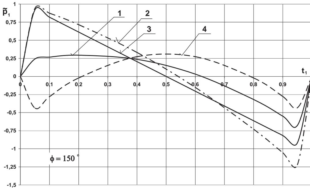
Fig. 1. Pressure distributions  $\tilde{p}_1$  in place  $\varphi=150^\circ$  in the time  $t_1$  by velocity perturbations: 1)  $V_{10}=0.05, V_{1h}=0$ , 2)  $V_{10}=0.05, V_{1h}=0.025$ , 3)  $V_{10}=0.05, V_{1h}=0.05$ , 4)  $V_{10}=0.05, V_{1h}=-0.05$
