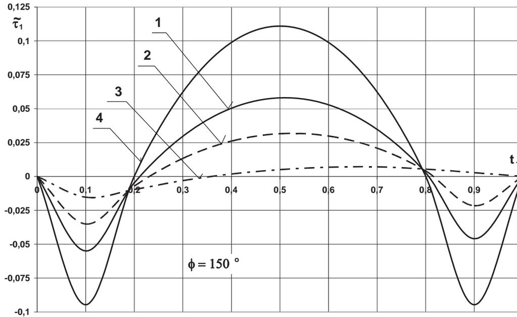
Fig. 4. Tangential pressure distributions  $\tilde{\tau}_1$  in place  $\phi=150^\circ$  in the time  $t_1$  by velocity perturbations: 1)  $V_{10}=0.05$ ,  $V_{1h}=0$ , 2)  $V_{10}=0.05$ ,  $V_{1h}=0.025$ , 3)  $V_{10}=0.05$ ,  $V_{1h}=0.05$ , 4)  $V_{10}=0.05$ ,  $V_{1h}=-0.05$
