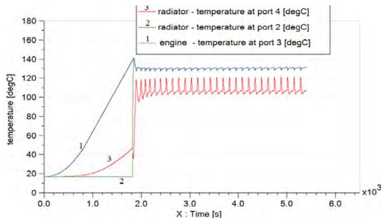
Fig. 4. Courses characteristic of the temperature at the pressure of 0.2 MPa and 33% of the filling with the liquid of the compensatory container for capacity 1.75 dm<sup>3</sup>: 1 – exit from the block of cylinders, 2 – entry to the radiator, 3 – exit from the radiator
