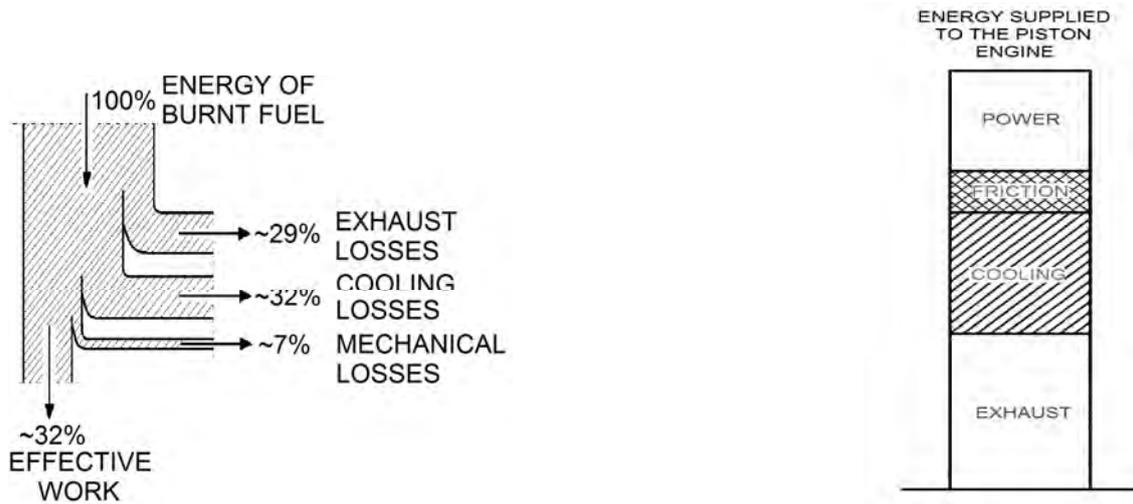
Fig. 1. Example of the heat balance of the piston internal-combustion engine [2, 12]
