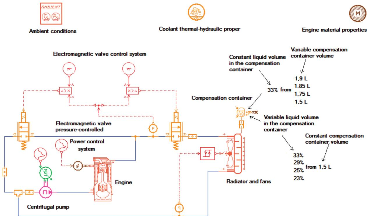
Fig. 3. The scheme of model stand of the cooling system developed in Amesim software
