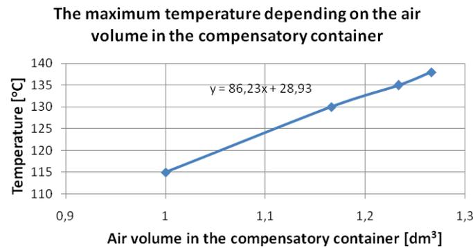
Fig. 7. Rise in temperature maximum in the function of the air volume in the compensatory container of the effect of increasing the volume of the container
