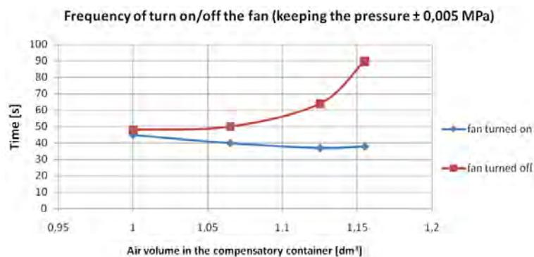
Fig. 9. Dependence of working hours of the fan after turn on liquid from the air volume in the compensatory container into results of reducing the number in the container
