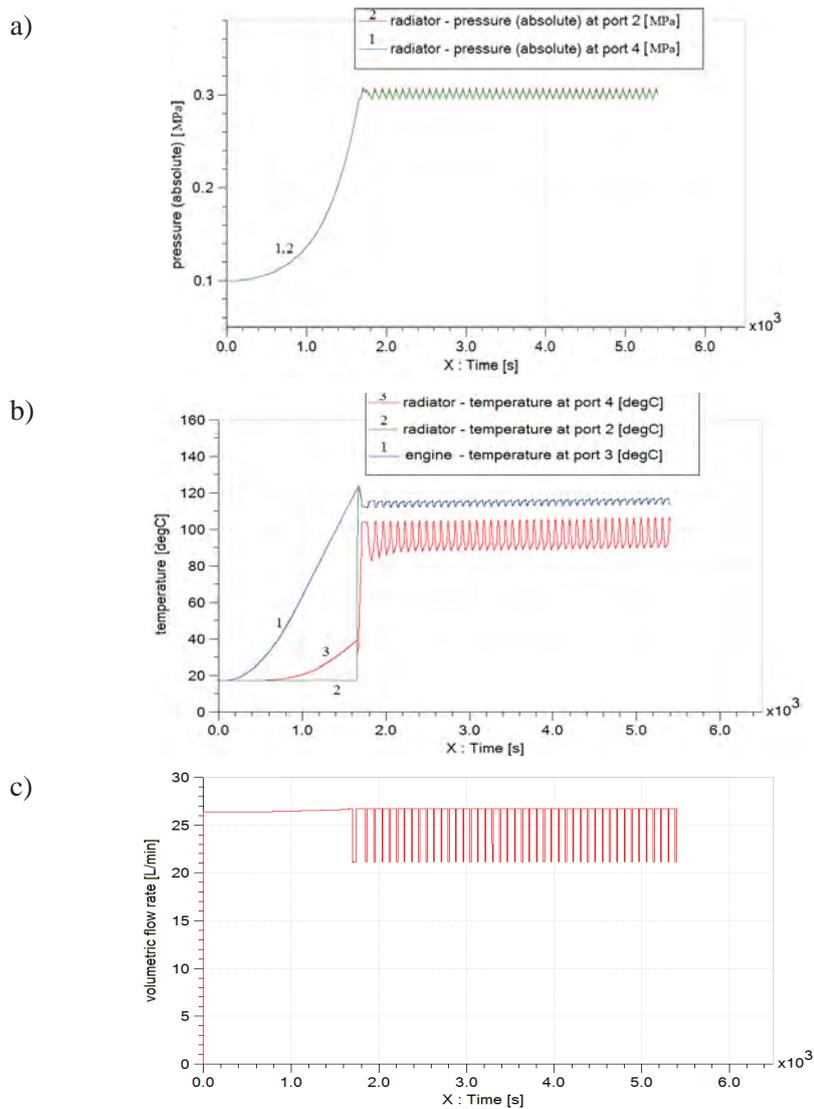
Fig. 3. Courses characteristics of chosen parameters of the simulated work of the cooling system at the pressure of 0.2 MPa and 33% of the filling up the compensatory container: a) course of the pressure: 1 – in the small circulation, 2 – in the large circulation, b) course of the temperature: 1 – exit from the block of cylinders, 2 – entry to the radiator, 3 – exit from the radiator, cooling c) course of the coolant pump flow
