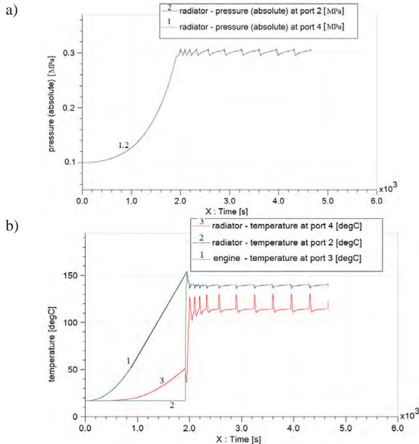
Fig. 5. Courses characteristics at the pressure of 0,2 MPa and 33% of filling up with coolant of the compensatory container for capacity 1.9 dm<sup>3</sup>: a) course of the pressure: 1 – in the small circulation, 2 – in the large circulation, b) course of the temperature: 1 – exit from the block of cylinders, 2 – entry to the radiator, 3 – exit from the radiator
