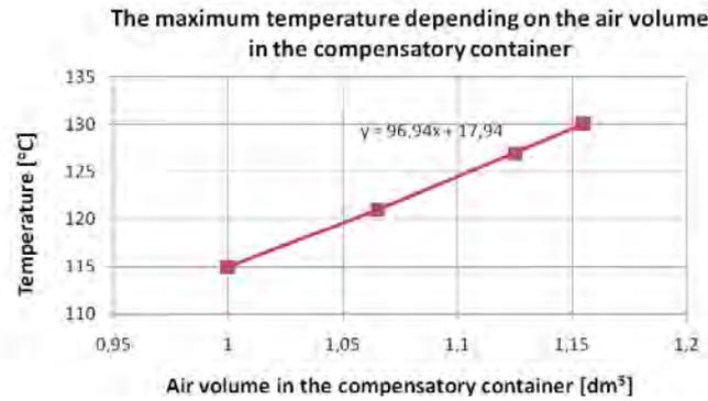
Fig. 6. Rise in temperature maximum in the function of the air volume in the compensatory container of the effect of reducing the number of liquid in the container
