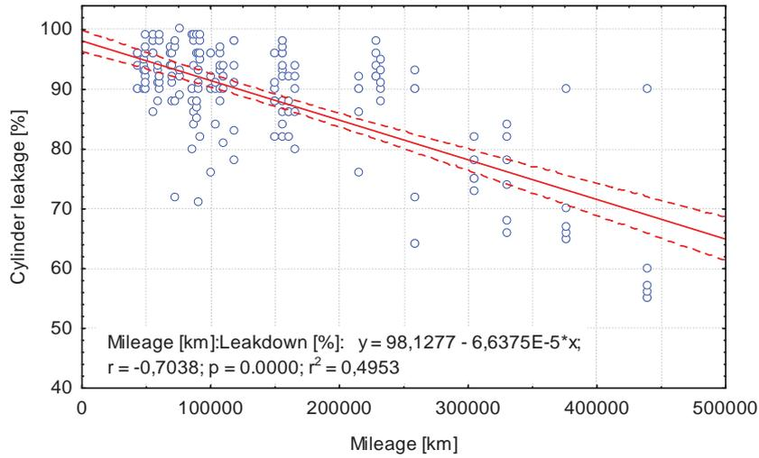
Fig. 2. Cylinder leakage as a function of mileage (a linear regression line and confidence area for the regression line at  $\alpha = 0.05$  were plotted)
