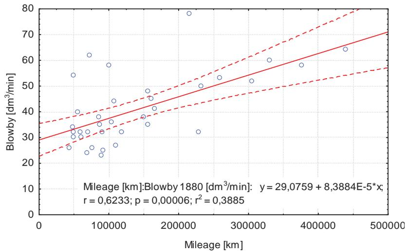
Fig. 5. Blowby rate at full engine load and rotational speed of 1880 rpm as a function of mileage (a linear regression line and confidence area for the regression line at  $\alpha = 0.05$  were plotted)
