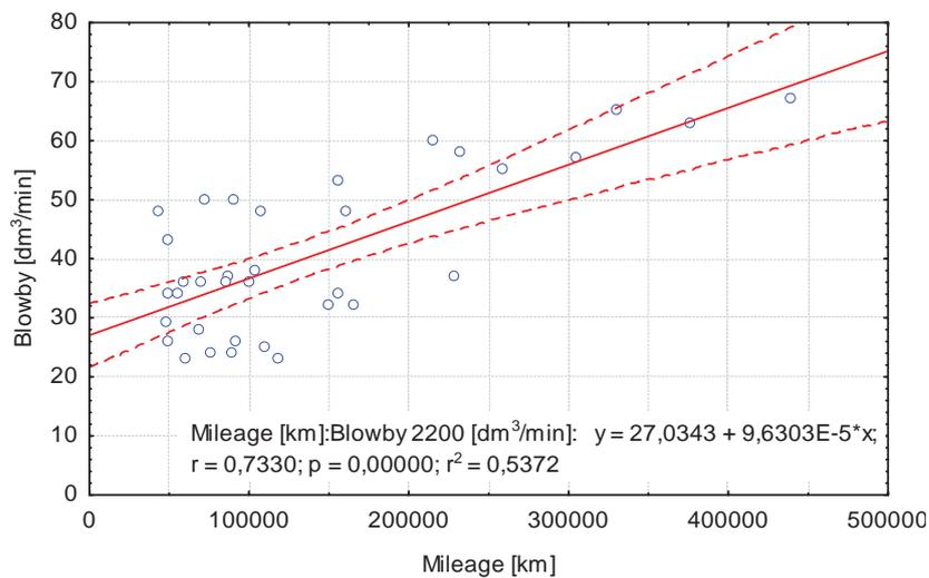
Fig. 6. Blowby rate at full engine load and rotational speed of 2200 rpm as a function of mileage (a linear regression line and confidence area for the regression line at  $\alpha = 0.05$  were plotted)
