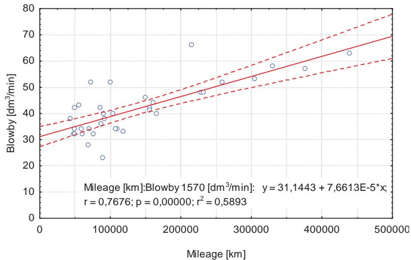
Fig. 4. Blowby rate at full engine load and rotational speed of 1570 rpm as a function of mileage (a linear regression line and confidence area for the regression line at  $\alpha = 0.05$  were plotted)
