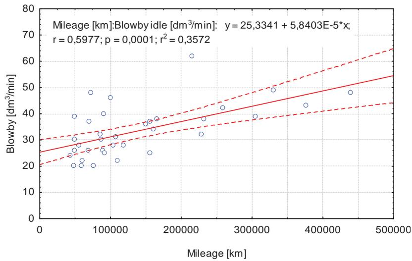
Fig. 3. Blowby rate at idle run as a function of mileage (a linear regression line and confidence area for the regression line at  $\alpha = 0.05$  were plotted)
