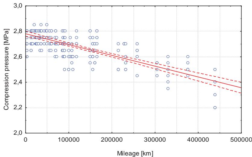
Fig. 1. Maximum compression pressure as a function of mileage (a linear regression line  $y = 2.791 - 8.761E-7*x$  and confidence area for the regression line at  $\alpha = 0.05$  determined for the measurement results obtained for mileages over 40,000 km)
