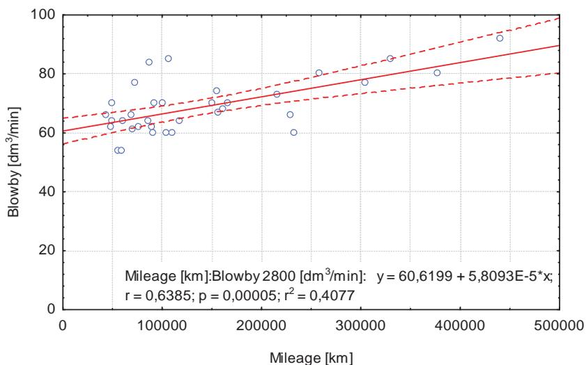
Fig. 7. Blowby rate at full engine load and rotational speed of 2800 rpm as a function of mileage (a linear regression line and confidence area for the regression line at  $\alpha = 0.05$  were plotted)
