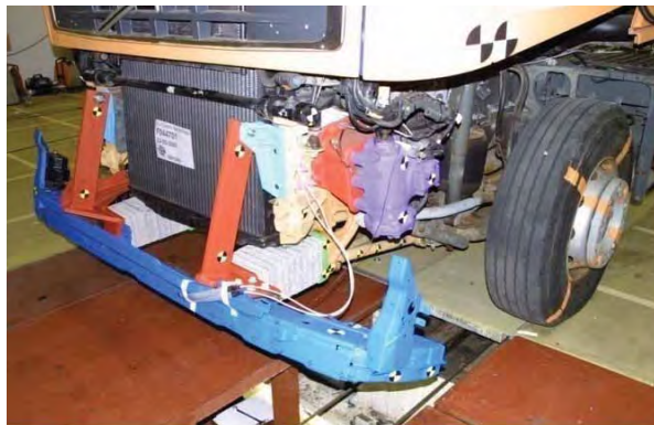
Fig. 5. Special kind of FUPDs with non rigid, aluminium foam blocks [7]
