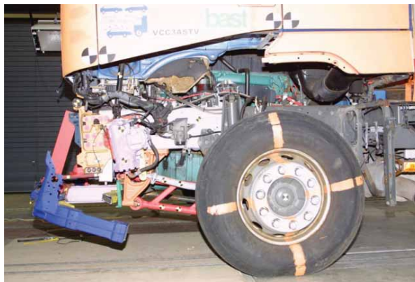
Fig. 6. Special kind of FUPDs with rigid, support brackets [7]
