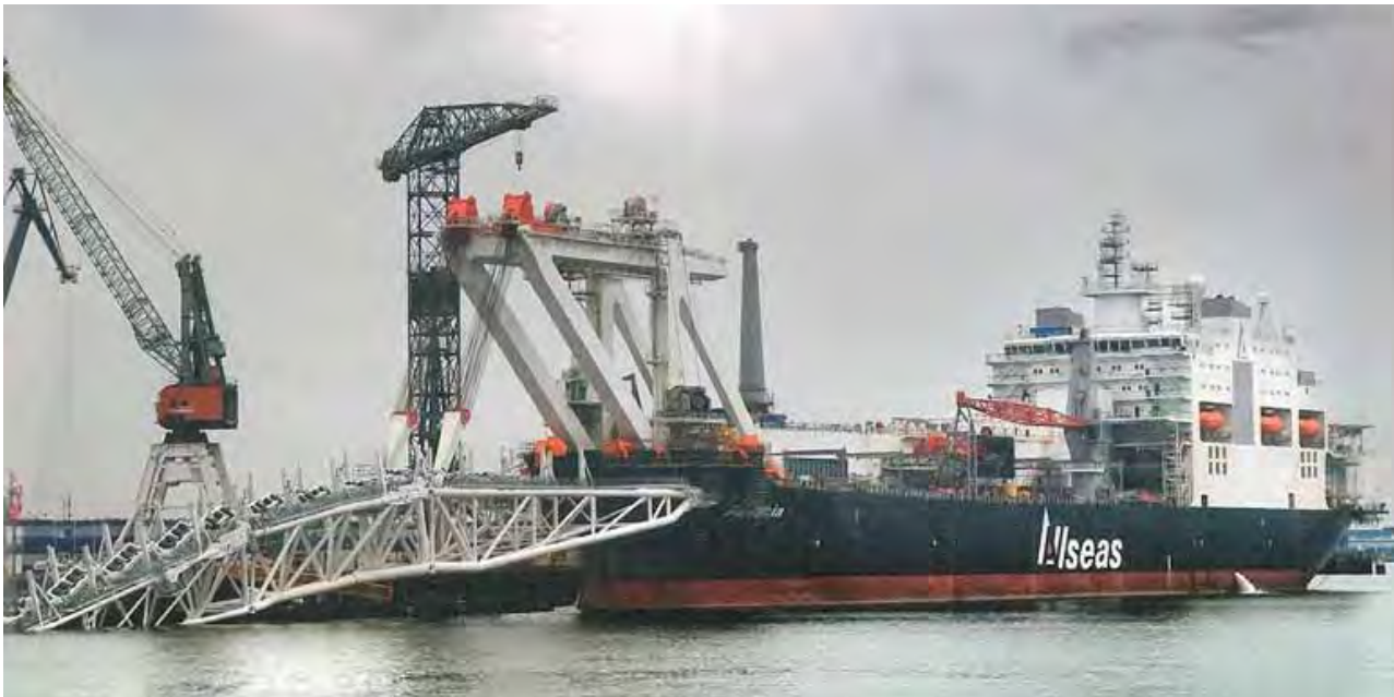
Fig. 2. Ms. Audacia – a bulkcarrier “Geeview” (built in 2005) converted (2007) into DP pipe-lay vessel [6]
