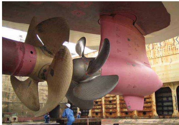
Fig. 1. Podded CRP propulsion is used in Hamanasu, built at MHI [2]
