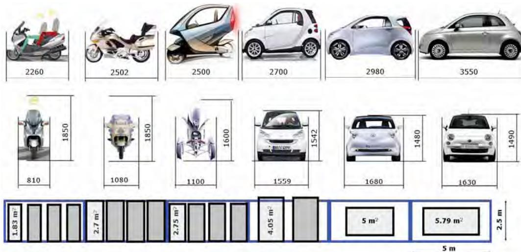
Fig. 2. Comparison of the space needed for parking PCV vehicles, small city vehicles, motorcycles and scooters [9]
