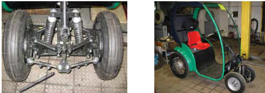
Fig. 6. Suspension with swivel axle [4]
