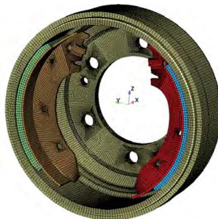
*Fig. 5. FE model of the brake*
