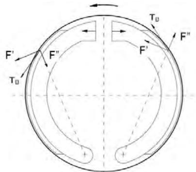
Fig. 2. Forces acting in SIMPLEX type drum brake [1]
