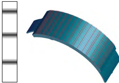
Fig. 6. Wearing pattern implemented in the „imperfect“ FE model
