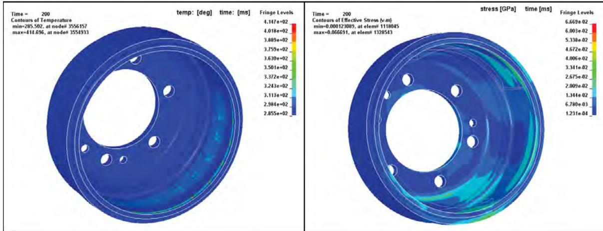
Fig. 10. Temperature and stress distribution in the drum for different times
