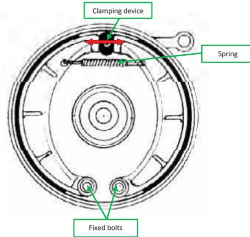
Fig. 1. SIMPLEX type drum brake
