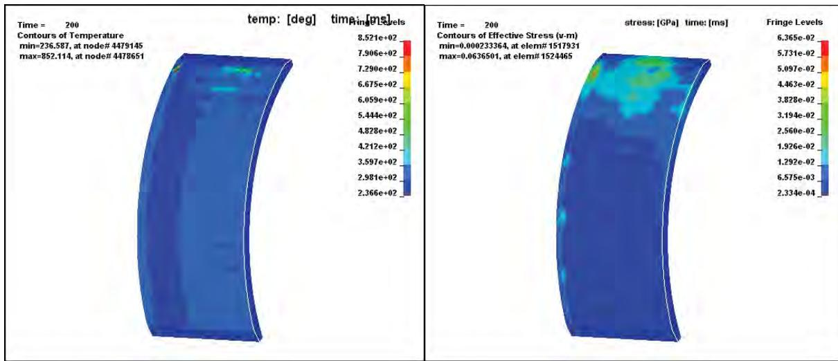
Fig. 11. Temperature and stress distribution in the shoe for different times
