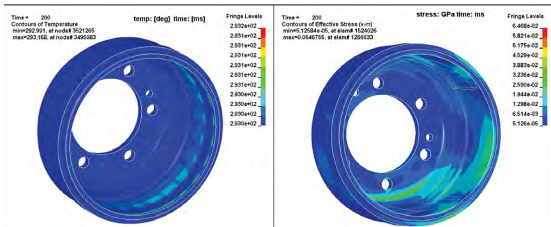
Fig. 7. Temperature and stress distribution in the drum for different times
