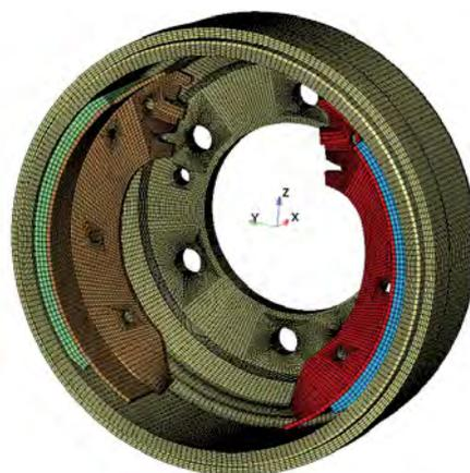
*Fig. 5. FE model of the brake*
