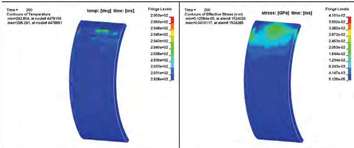
Fig. 8. Temperature and stress distribution in the shoe for different times
