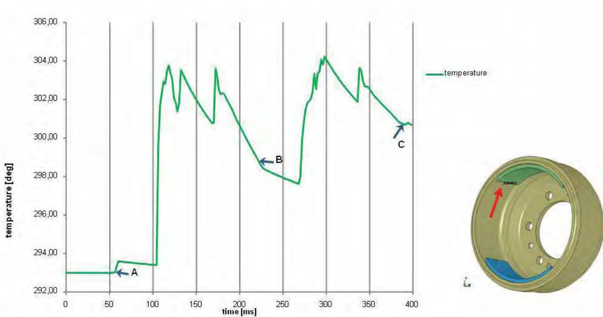
Fig. 12. Temperature generation based on the contact model
