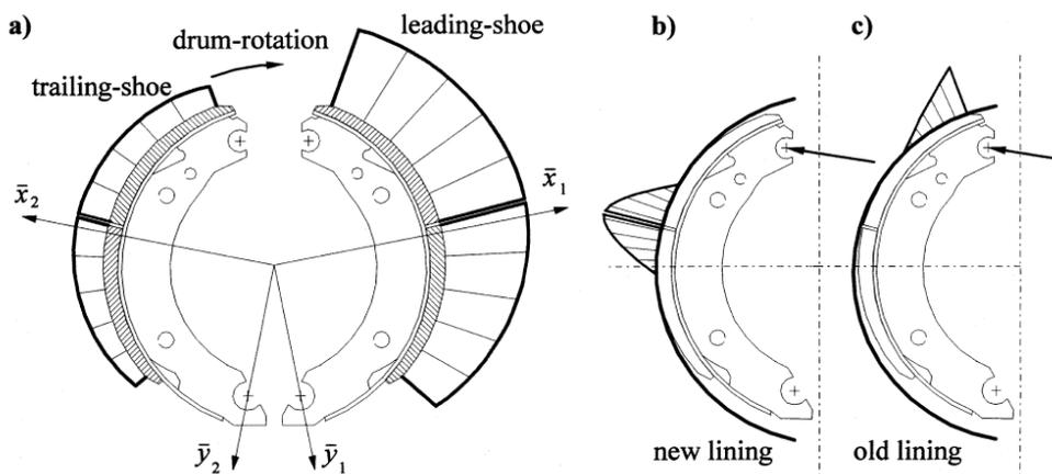
Fig. 3. Normal pressure distribution assumed by Koessler (a), for a new (b) and an old lining (c) [1]
