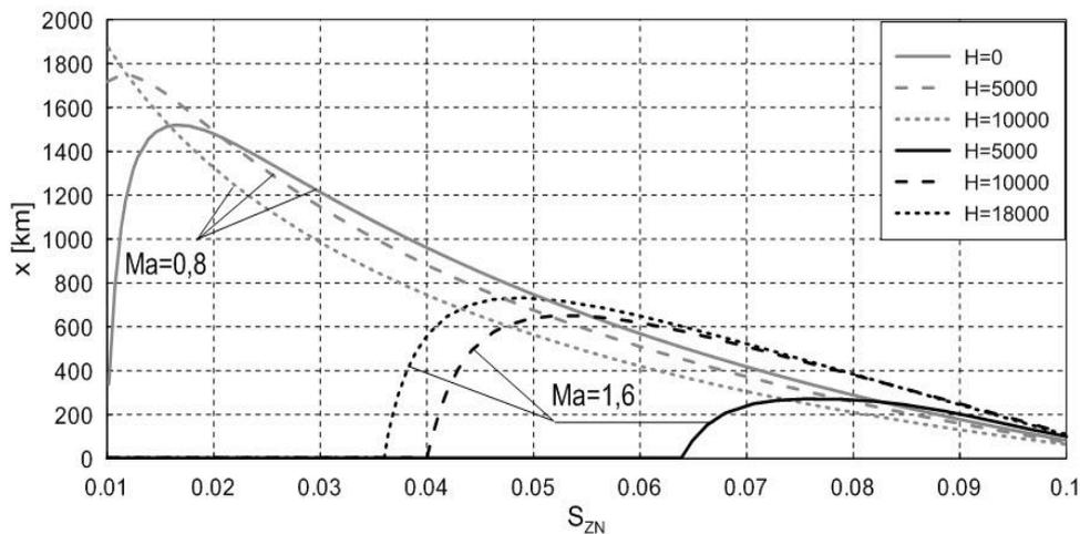
Fig. 2. Influence of  $S_{ZN}$  and flight conditions ( $Ma, H$ ) on theoretical range
