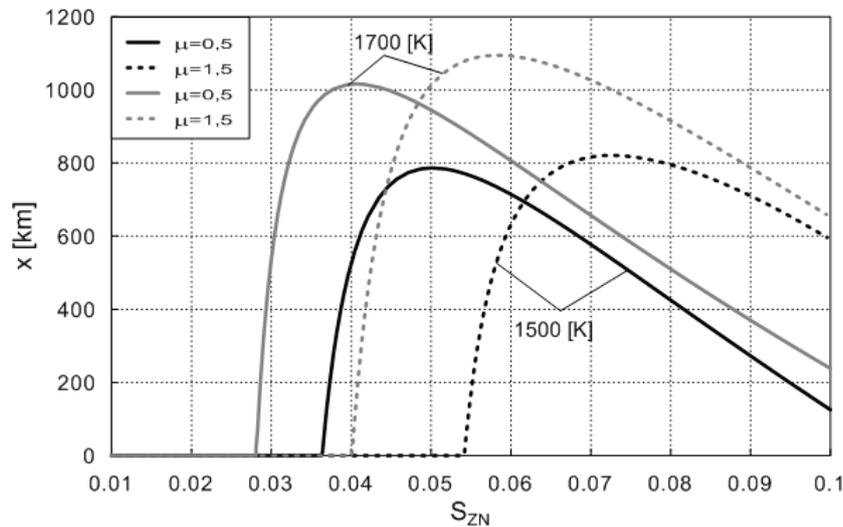
Fig. 5. Influence of bypass ratio  $\mu$  and temperature before turbine  $T_3$  and change  $S_{ZN}$  on the range  $x$  for the supersonic flight ( $Ma=1.6, H=18000\text{ m}$ )
