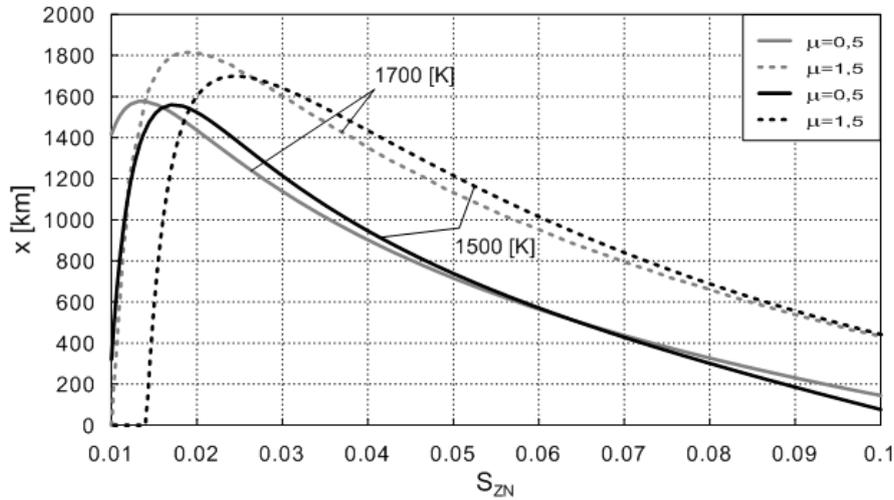
Fig. 4. Influence of bypass ratio  $\mu$  and temperature before turbine  $T_3$  and change  $S_{ZN}$  on the range  $x$  for the subsonic flight ( $Ma=0.8, H=0$ )
