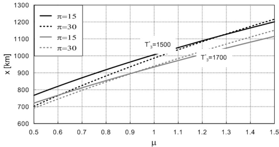
Fig. 6. Influence of engine cycle parameters on the range  $x$  (subsonic flight)
