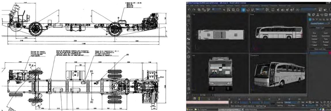
*Fig. 1. Typical bus chassis frame available from authorized distributor(left) and drawings of bus exterior (right)*
