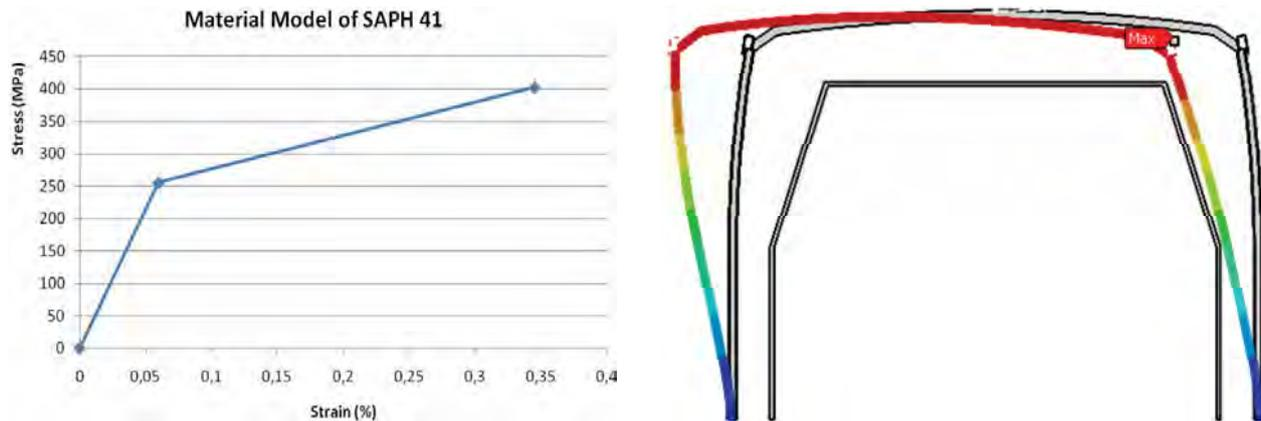
Fig. 8. Material model (left) and plastic deformation of finite element model of body section (right)
