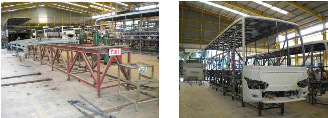
*Fig. 2. A body assembling fixture (left) and a completed bus superstructure (right)*
