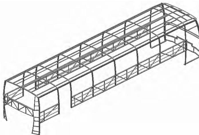
Fig. 3. Computer drawing of bus superstructure (floor framework not shown)
