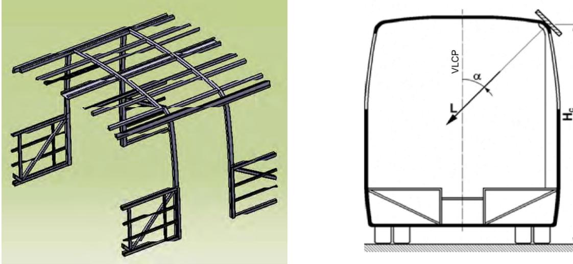
Fig. 7. Geometric model of a section of superstructure (left) and direction of quasi static load (right)
