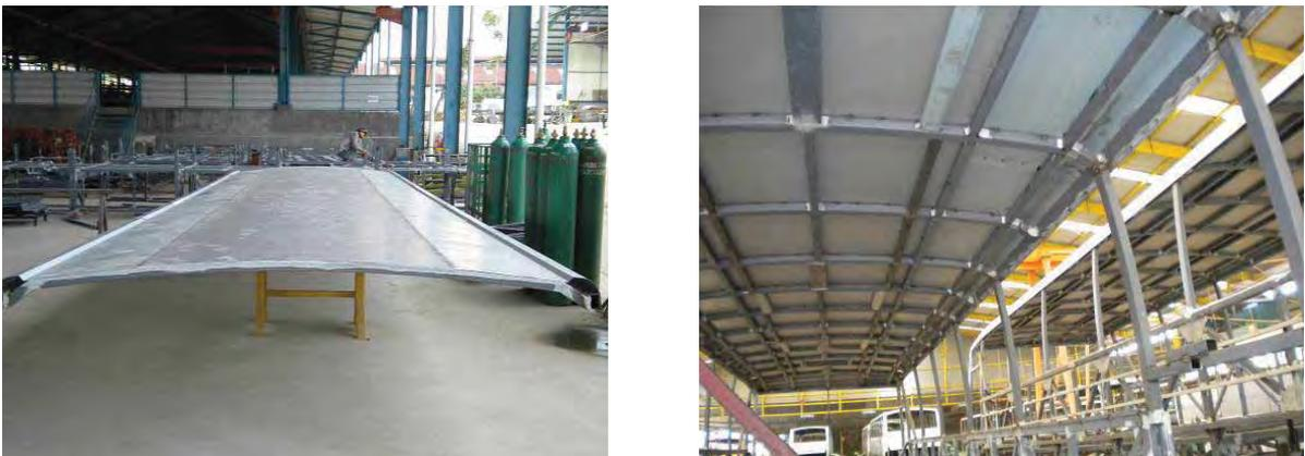
Fig. 5. A roof framework (left) and a completed superstructure (right)
