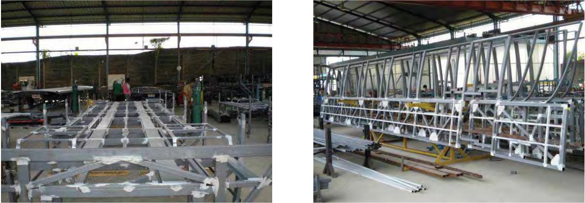
Fig. 4. Floor frame (left) and body side frame (right)
