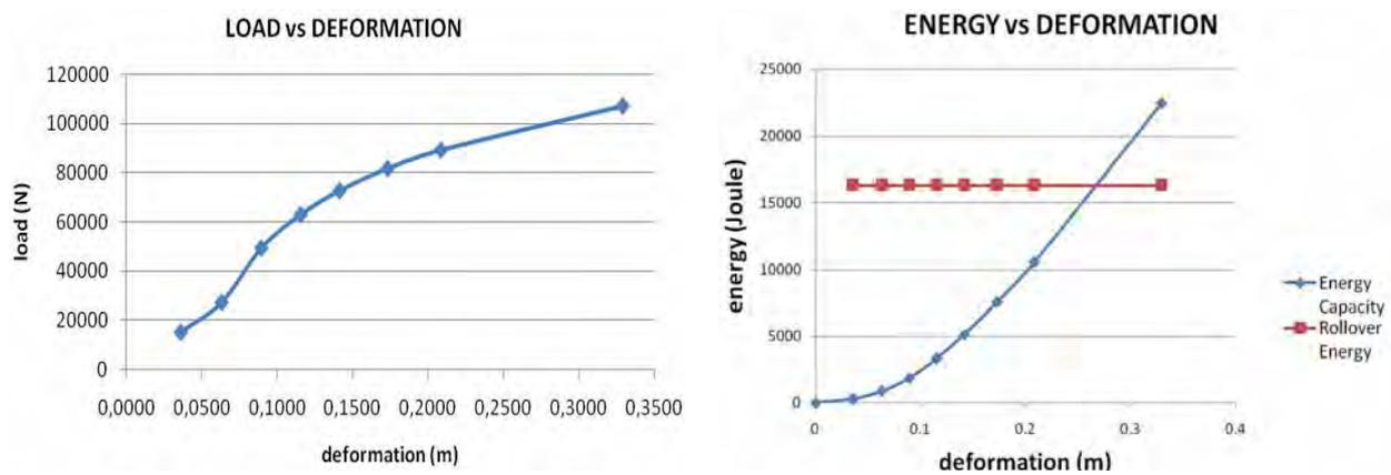
Fig. 9. Load vs. deformation (left) and energy vs. deformation (right)
