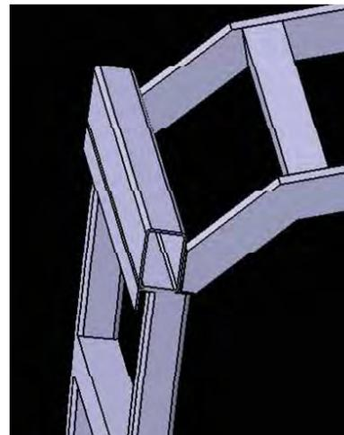
Fig. 6. Details of joint between pillar and roof bow
