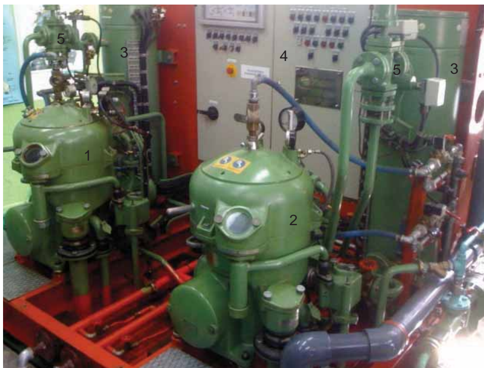
Fig. 2. The view of the WESTFALIA purifiers test stand: 1 - lubricating oil centrifuge working in UNITROL system, 2 - lubricating oil centrifuge working in SECUTROL system, 3 - electric heater, 4 - control panel, 5 - three-way valve
