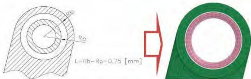
Fig. 8. Revolute joint radial clearance introduced to the landing gear model
