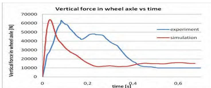
Fig. 5. Wheel axle vertical force-time diagram
