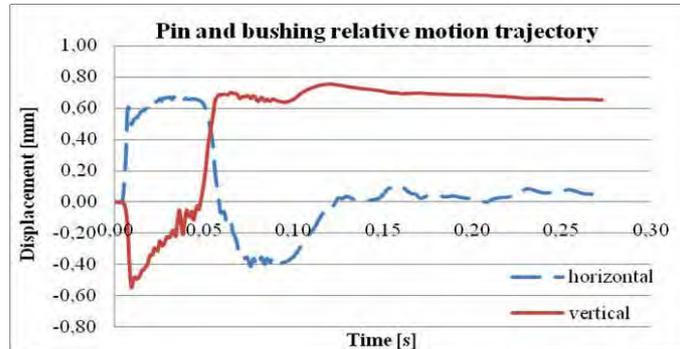
Fig. 9. Pin and bushing relative motion trajectory for 0.75 [mm] radial clearance case
