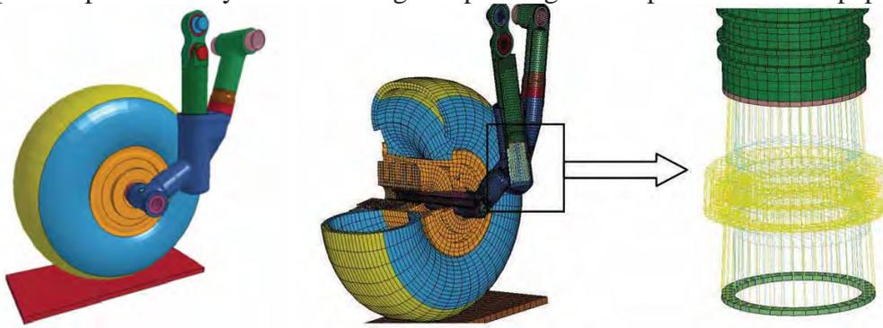
Fig. 6. Complete landing gear geometrical and FE model with the gear shock absorber discrete model
