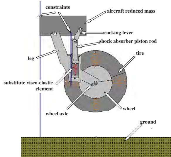
Fig. 4. Two-dimensional model developed in MSC Working Model [4]
