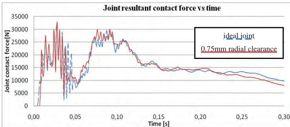
Fig. 10. Revolute joint resultant contact force-time graph
