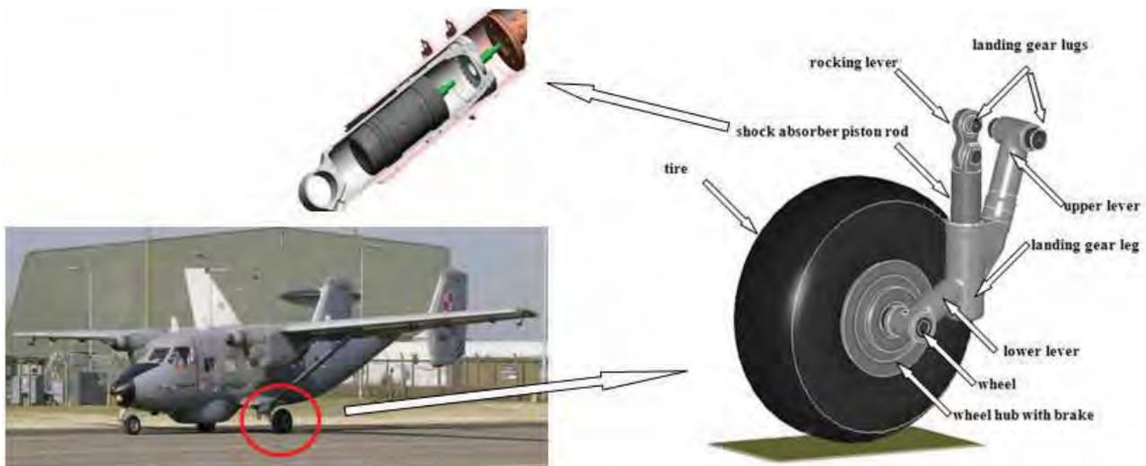
Fig. 3. PZL M28B Bryza and the investigated landing gear main components
