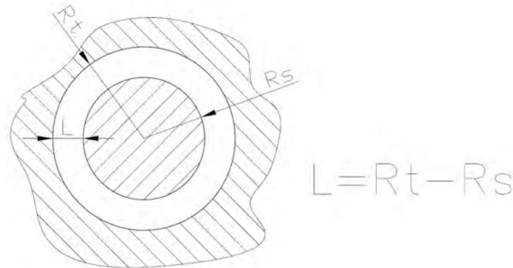
Fig. 1. Radial clearance in a pin joint
