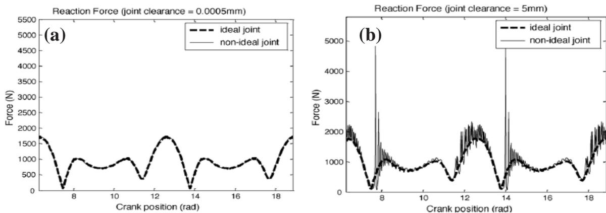
Fig. 2. The dependence of reaction force in a joint on crank position (time) [7]
