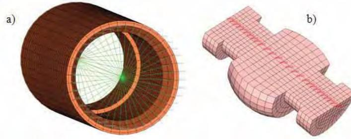
Fig. 7. Mass elements connection to upper lever pin (a) and rocking lever (b)
