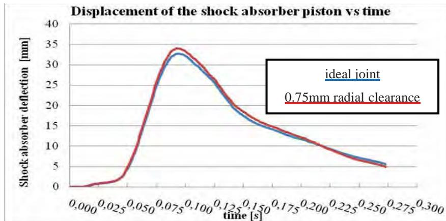
Fig. 12. Shock absorber deflection-time diagram comparison for considered cases
