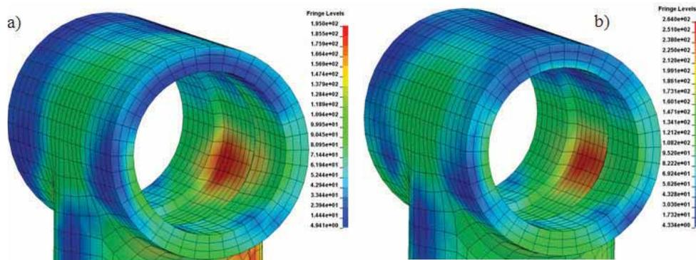
Fig. 11. von Mises stress fringes in the joint bushing zone for: (a) the ideal joint case (max 195[MPa]) and (b) 0.75[mm] clearance mode (max 264[MPa]) after 0.034[s] of drop tests time
