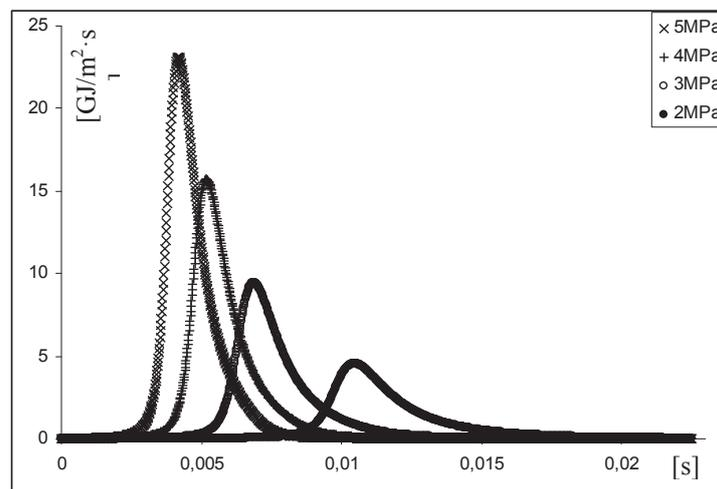
Fig. 1. The example of the kinetic calculation effects of heat release from combustion process in temperature 1100 K, humidity of air 10 g water on 1kg of air and air-fuel excess ratio equals 0,8
