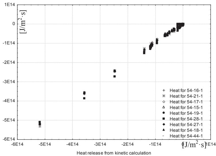
Fig. 4. The best ANN approximations of the kinetic calculations of the heat release for all considered parameters of the combustion process
