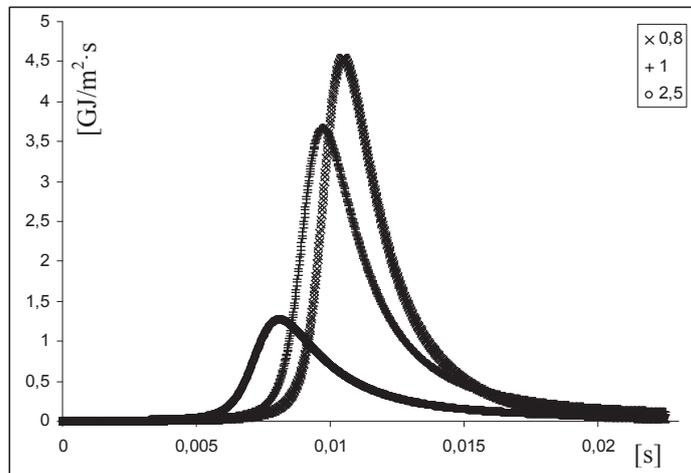
Fig. 3. The example of the kinetic calculation effects of the heat release from combustion process in temperature 1100K, pressure 2MPa humidity of air 10g water on 1kg of air
