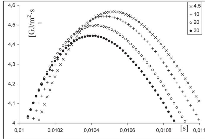
Fig. 2. The example of the kinetic calculation effects of the heat release from combustion process in temperature 1100K, pressure 2MPa and air-fuel excess ratio 0.8
