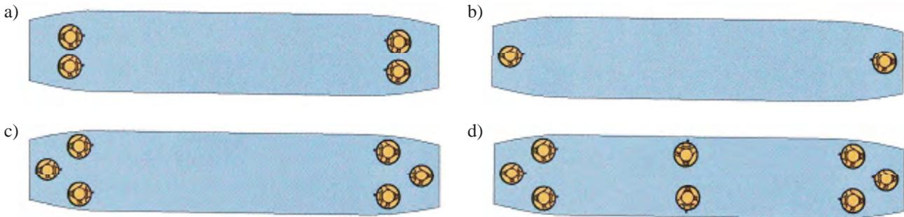
Fig. 1. Possibilities of multi-element propulsion arrangement for DP systems: a) the most popular, b) the minimum, c) good for DP, d) full possibilities
