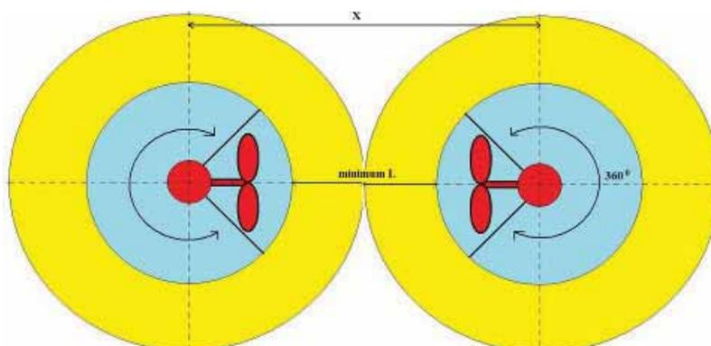
Fig. 3. Minimum distance "L" between nozzleed thrusters
