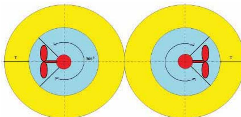
Fig. 4. Zero thrust position – the thrusters work at the same conditions and parameters
