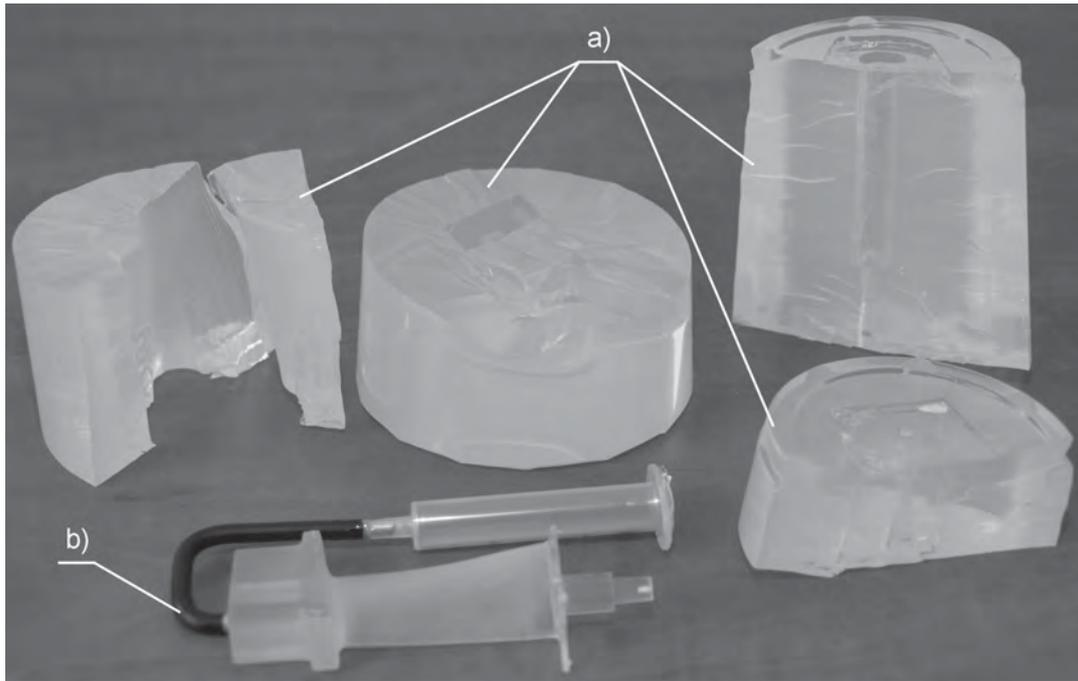
Fig. 4. Silicone mold (a) manufactured on the basis model kit (b)
