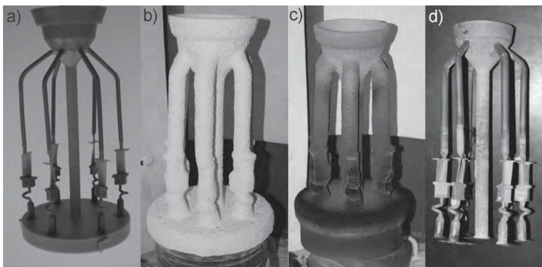
Fig. 6. Application of wax models to manufacturing of monocrystal blades: a) wax model kit, b) ceramic form before casting, c) form in the stove after casting, d) monocrystal blades
