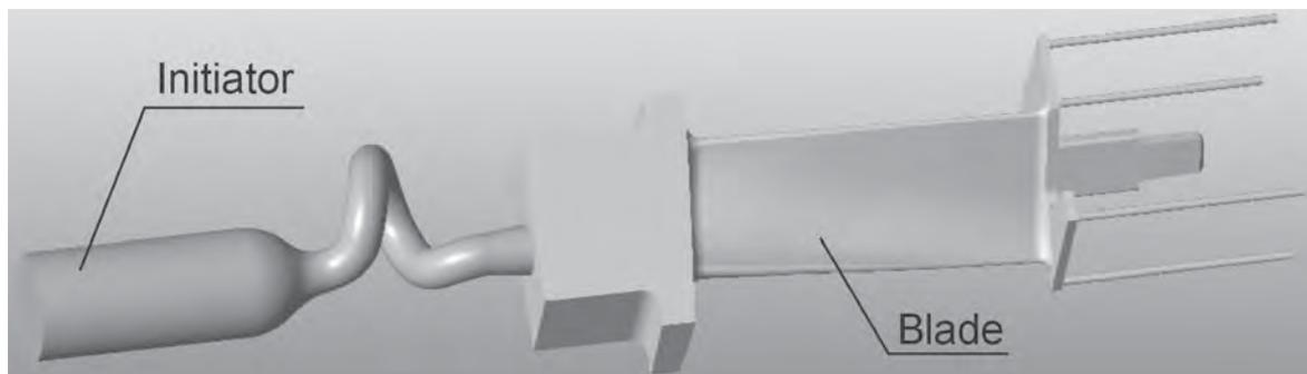
Fig. 1. Model CAD of blade and also initiator
