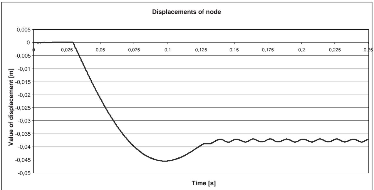
Fig. 12. Diagram presenting displacements of monitored node in a yielding support
