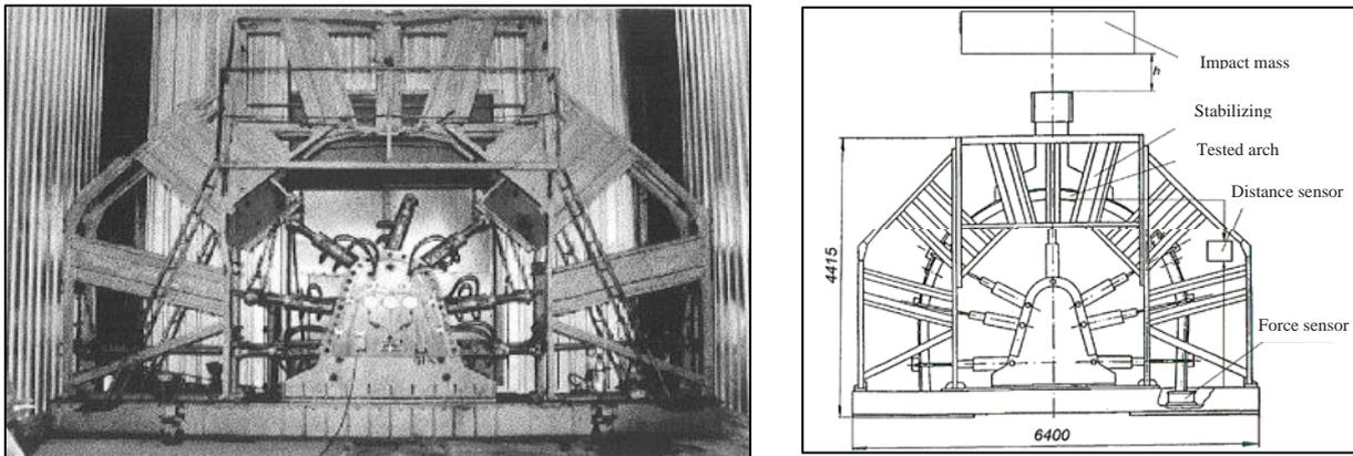
Fig. 7. Stand for testing a frame of arch supports used at the Central Mining Institute in Katowice
