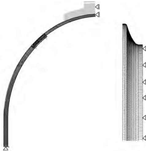
Fig. 4. Boundary conditions and position of contact places in the calculation model
