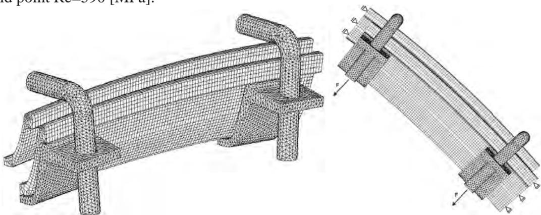
Fig. 9. Computational model for static analysis – screwing together the support's arches
