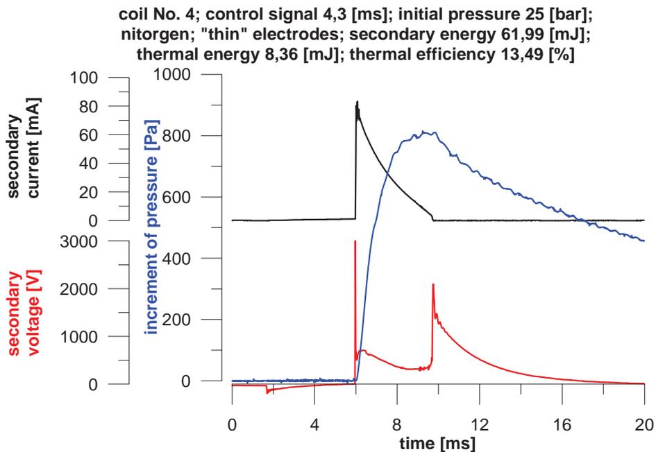
Fig. 3. Pressure increment in the chamber, secondary voltage and secondary current in the coil No. 4 at initial pressure of 25 bar for spark plug with “thin” electrodes
