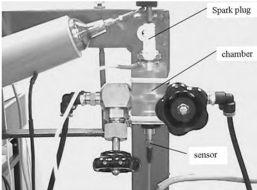
Fig. 2. Measurement chamber with needle valves, pressure sensor and spark plug
