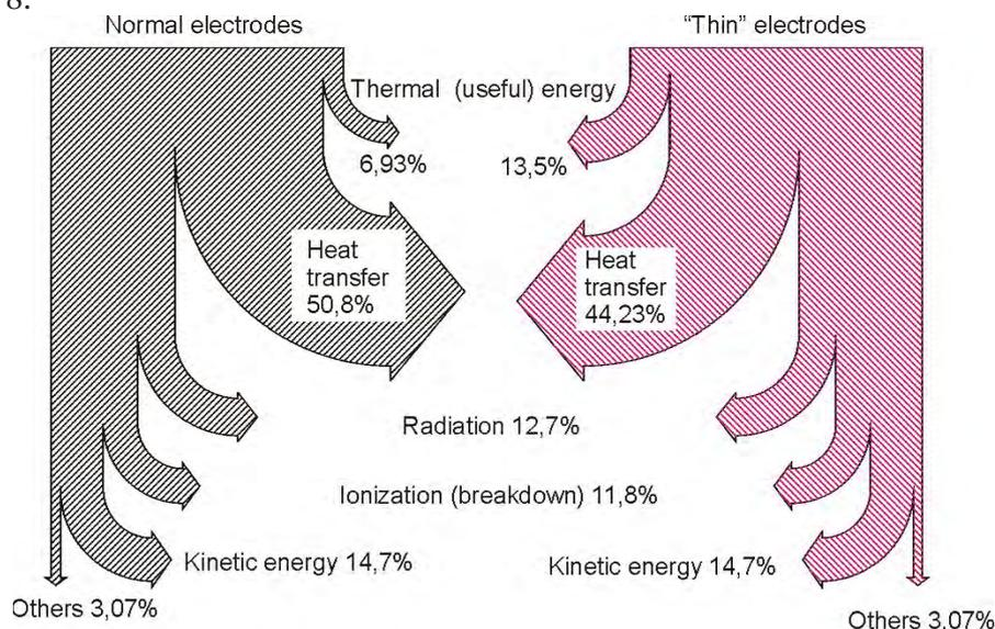
Fig. 8. Balance of energy in a conventional ignition system for two types of electrodes
