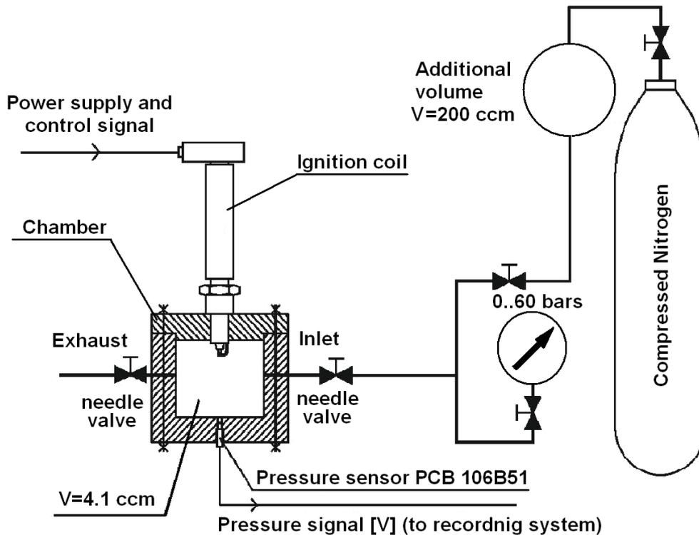
Fig. 1. Scheme of the direct pressure measurement method in the caloric chamber
