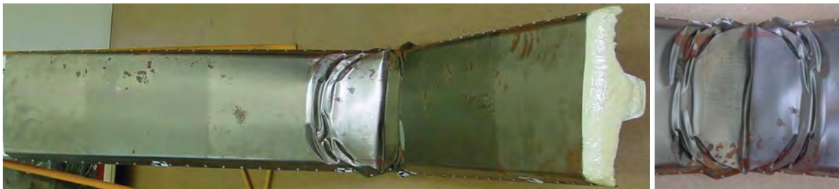
Fig. 3. Protection panel after a carried out test according to the I load variant
