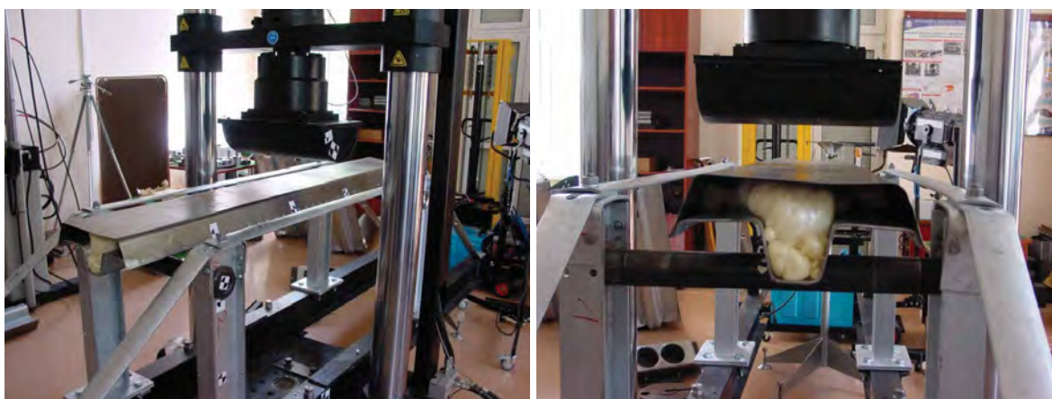
Fig. 1. Examination stand for the three point bending test at the traverse angle of incidence 90° - with a protection panel
