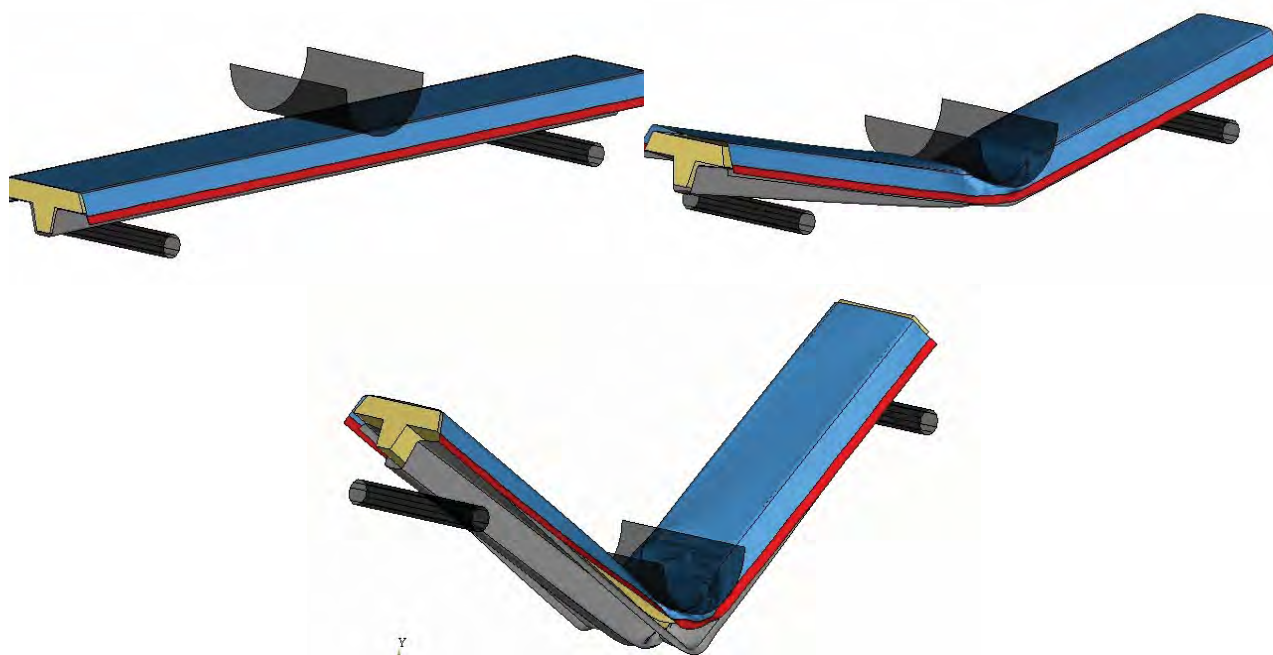
Fig. 6. Numerical simulation of the protection panel bending test on the test stand at the traverse angle of incidence 90^\circ . Figures show numerical deformation of the model by the traverse displacement in succession: 0; 200 and 450 mm
