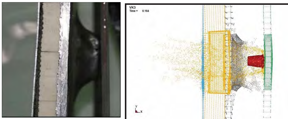
Fig. 7. Perforation of the selected structure of the panel, experiment (left), simulation (right)
