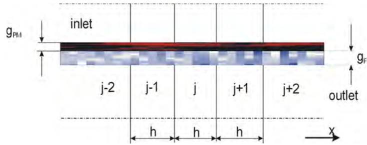
Fig. 3. Numerical scheme of the calculation mesh along the channel's length
