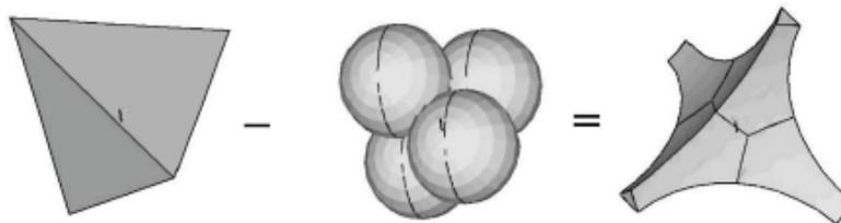
Fig. 4. A tetrahedron and spheres to generate a unit cell of a foam[6]
