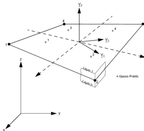
Fig. 7. Form of the bilinear thin-shell element
