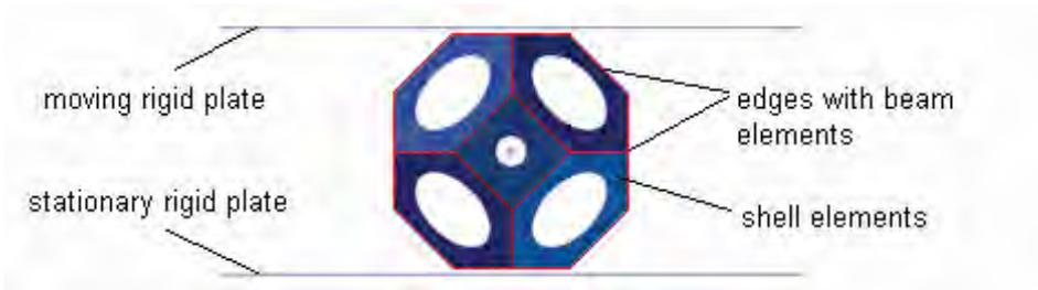
Fig. 6. The numerical model – finite elements and boundary conditions
