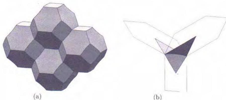
Fig. 2. Four cells in the Kelvin foam (a), and one fundamental piece (b), consisting of a fourth of one square and sixths of two hexagons, the region near a particular triple edge
