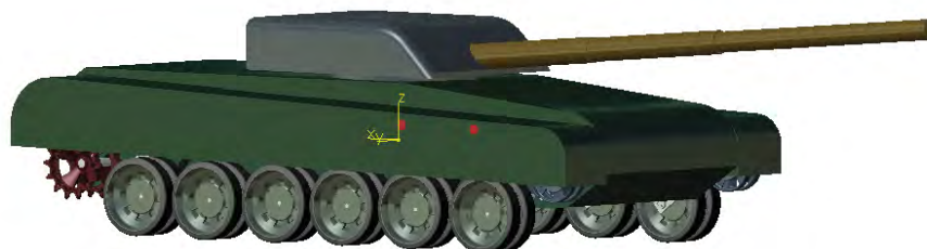
Fig. 3. Assemblage of all CAD model elements of the tank including suspension
