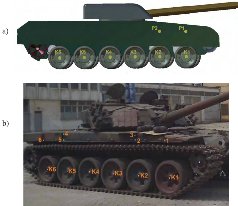
Fig. 9. Distribution of points on the body and wheels axes: a) model, b) the real object
