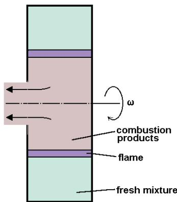
Fig. 9. Side view of flame propagating in a rotating cylindrical combustion chamber shown in a form of schematic diagram
