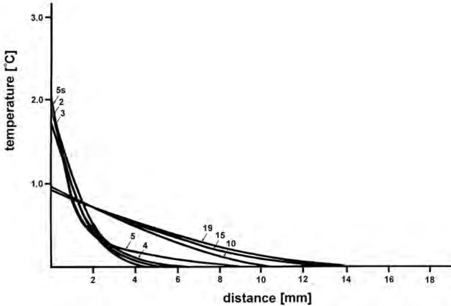
Fig. 8. Calculated temperature profiles inside the rod for lean limit downward propagating flame (6%CH<sub>4</sub>)
