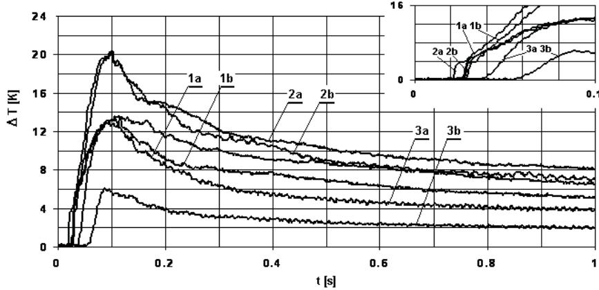
Fig. 13. Measured profiles of temperature changes in the combustion chamber wall surface. Methane/air mixture 8.45%CH<sub>4</sub>; 1a, 1b - T<sub>1</sub>, T<sub>2</sub>, rotational speed 1000rpm, 2a, 2b, - T<sub>1</sub>, T<sub>2</sub>, rotational speed 3000rpm, 3a, 3b, - T<sub>1</sub>, T<sub>2</sub>, rotational speed 5000rpm (in right top edge of the figure initial part of temperature rise is shown in detail)
