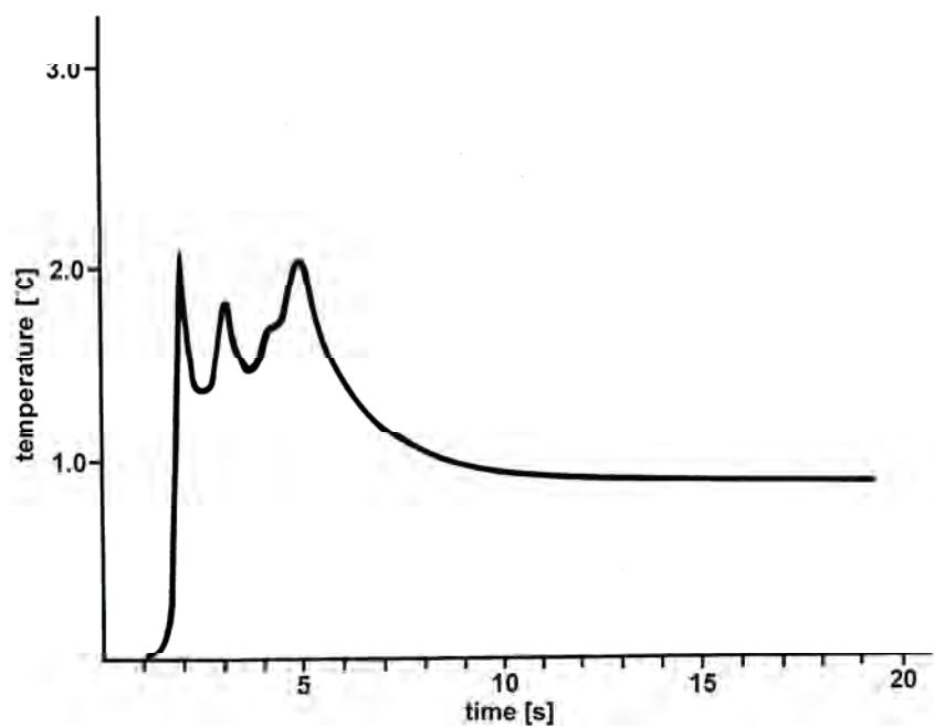
Fig. 5. Example of wall surface temperature record for lean limit methane/air mixture (6%CH<sub>4</sub>)
