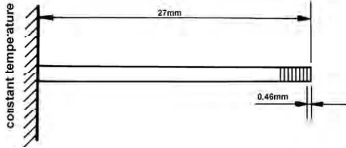
Fig. 6. Mullit rod considered as a one-dimensional system subdivided for numerical solution. Rod is 27 mm long. Calculations were performed for a 46 mm rod. Calculations showed that heat pulse applied at right end did not penetrate 27 mm in 20 second-the test time
