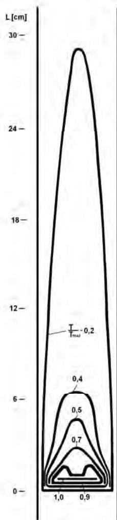
Fig. 4. Flame thermal structure. Isotherms determined based on temperature curves indicated in Fig. 3 (with assumption of axial symmetry)
