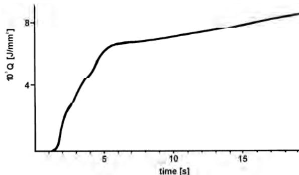
Fig. 7. Calculated heat transfer to the gauge from lean limit downward propagating flame (6%CH4)
