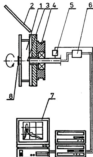
Fig. 10. Experimental set-up: 1-cylindrical chamber (with venting orifice in axis of rotation), 2-mirror, 3-ignitor, 4-V-belt wheel, 5-solenoid valve, 6-mixture supply, 7-PC, 8-tissue paper on the outflow orifice
