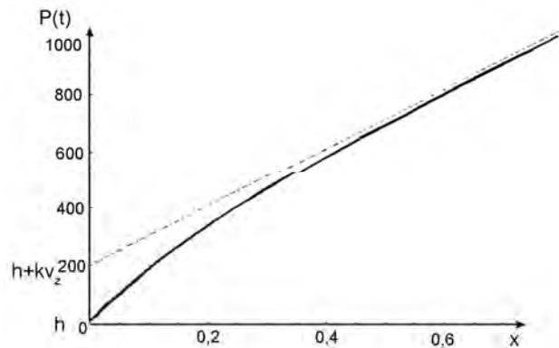
Fig. 7. Graphical representation of the relation (10) for an analysis of quasi-static penetration
