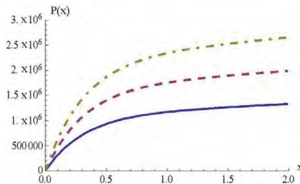
Fig. 3. Quasi-static characteristics for various  $i$  impact velocities: (solid line -  $v_0=10\text{m/s}$ , dashed line -  $v_0=15\text{m/s}$ , dash-dot line -  $v_0=20\text{m/s}$ )
