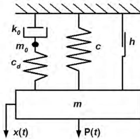
Fig. 6. Zener type degenerated model with dry friction
