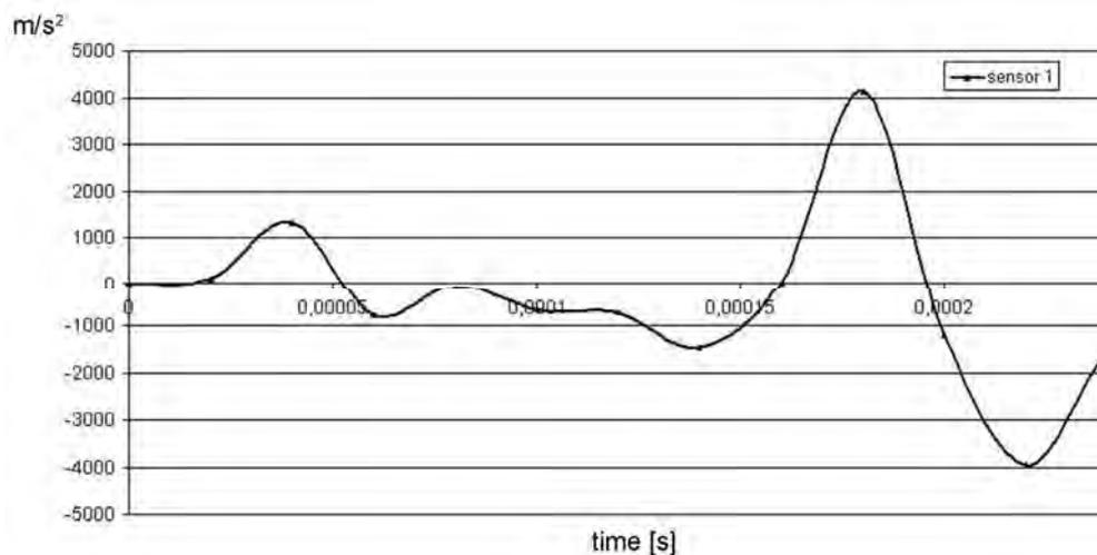
Fig. 12. The acceleration registered by the sensor No.1 during impact of 9 mm Parabellum bullet with impact velocity 358 m/s
