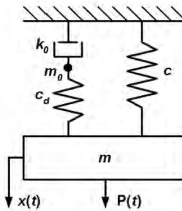
Fig. 1. Selected degenerated model with viscotie suppression
