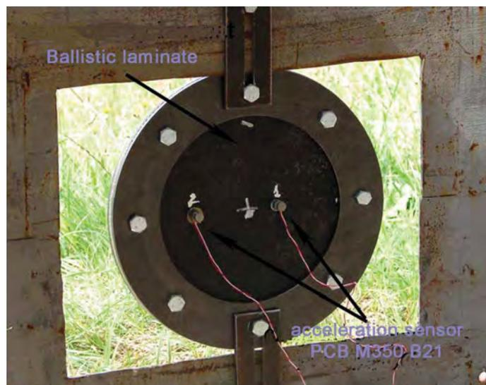
Fig. 10. Experiment station of punching the ballistic shield
