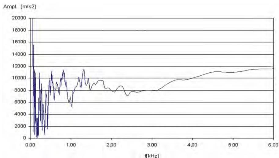
Fig. 13. Frequency characteristic during impact of 9 mm Parabellum bullet with impact velocity 358 m/s
