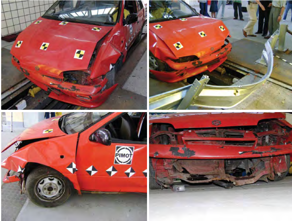
Fig. 8. Suzuki Swift car's deformation
