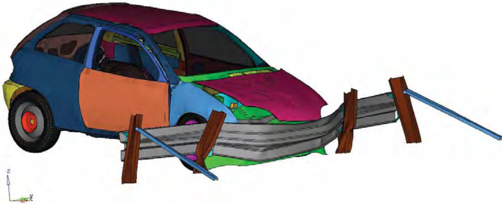
Fig. 13. Car-guardrail system at the instant t=0.3 s
