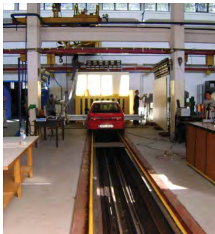
Fig. 1. Stand for vehicle crash tests with a barrier in PIMOT's Vehicle Safety Laboratory
