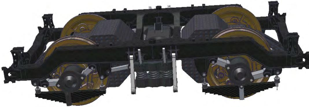
Fig. 2. CAD model of wheel bogie
