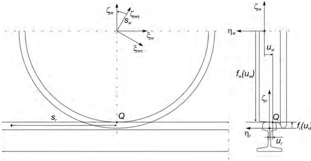
Fig. 4 The parameters used to describe the wheel and rail surfaces
