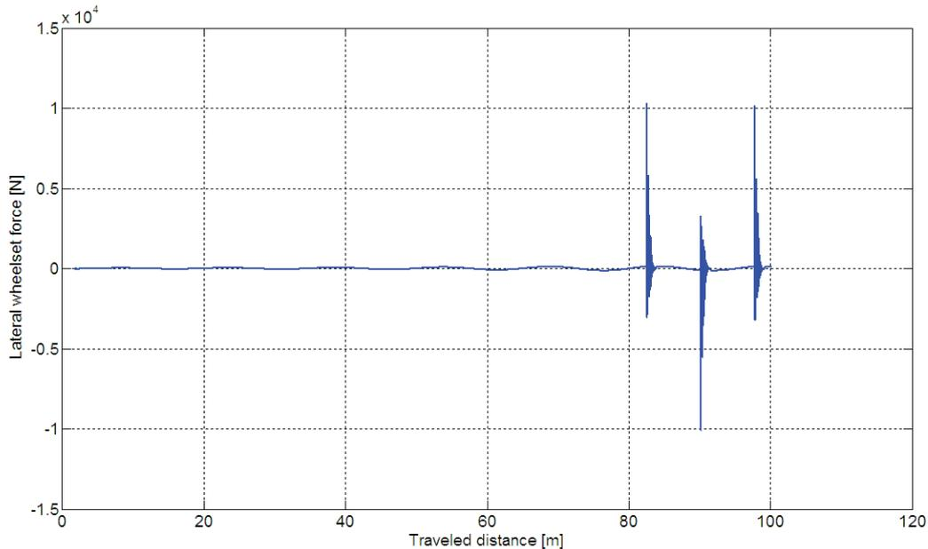
Fig. 7. Lateral contact force on wheelset for a forward velocity of 10 m/s
