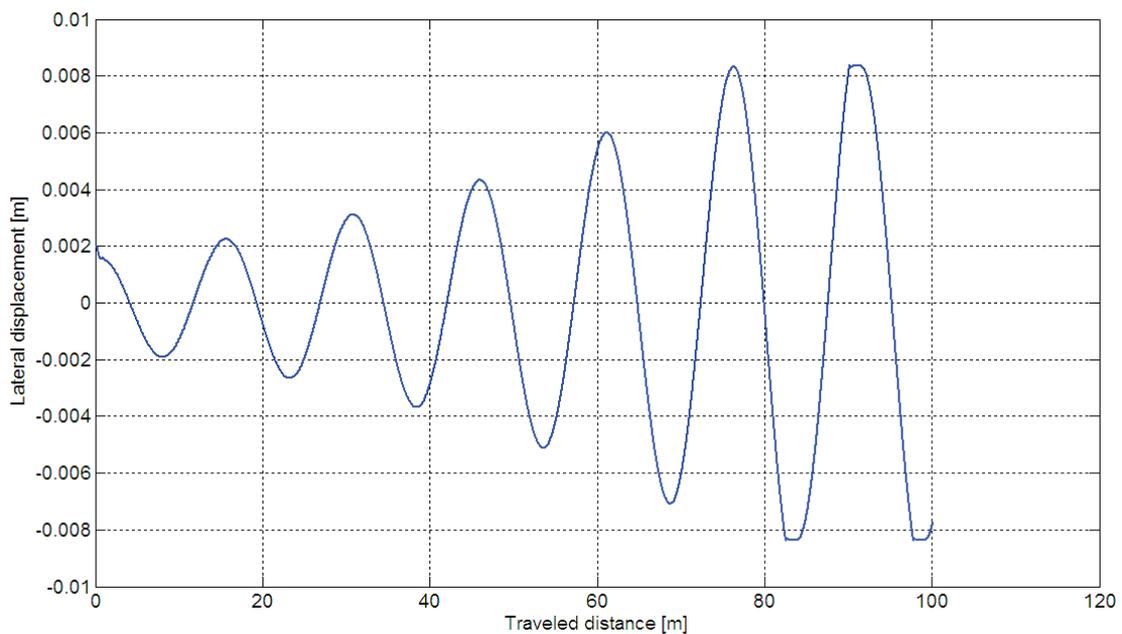
Fig. 6. Lateral displacement of the vehicle wheelsets for a forward velocity of 10 m/s
