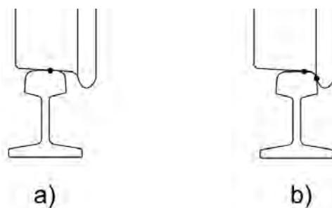
Fig. 8. Different types of contact between wheel and rail: a) tread contact – one point of contact; b) flange contact – two points of contact
