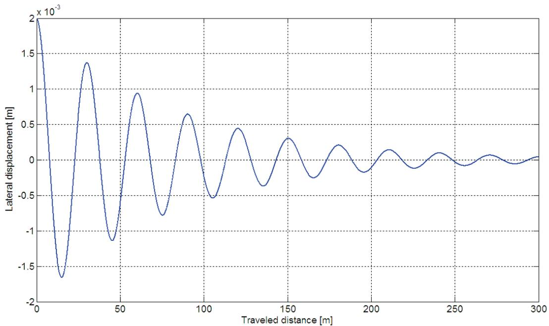
Fig. 5. Lateral displacement of the front wheelset for vehicle forward velocity of 10 m/s
