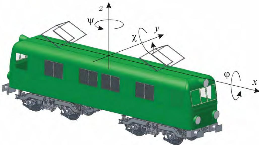
*Fig. 1 Model of the vehicle created in Inventor program*
