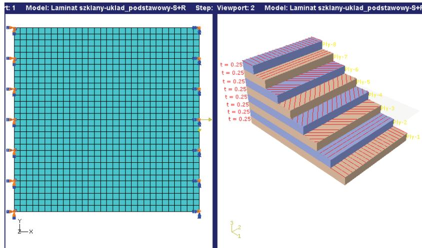
Fig. 1. Discrete numerical model of composite plate for quasi-isotropic system
