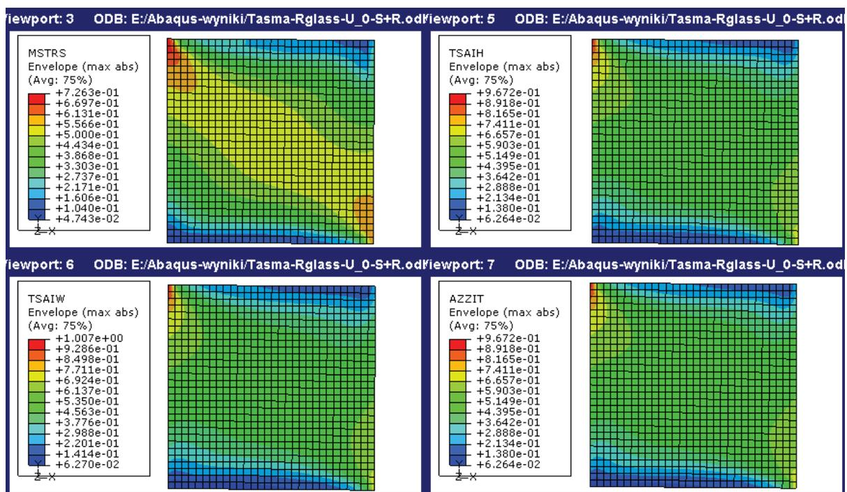
Fig. 2. The composite effort of  $[0]_8$  system in all layers: (a) the Maximum Stress Criterion, (b) Tsai-Hill's criterion, (c) Tsai-Wu criterion, (d) Azzi-Tsai-Hill's criterion
